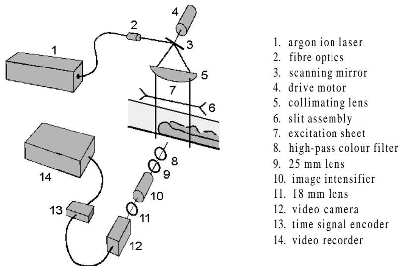
Fig. 4. Schematic of the flow illumination and image acquisition systems used to visualize small-scale gravity currents.
