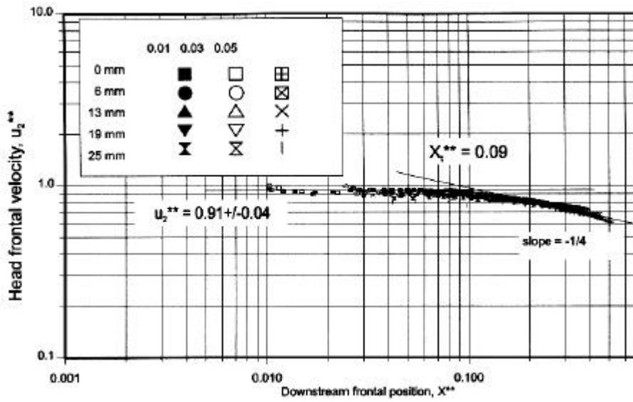
Fig. 7. Head frontal velocity versus downstream position for all gravity current flows over the range of surface roughness scale and source fluid density excess used.
