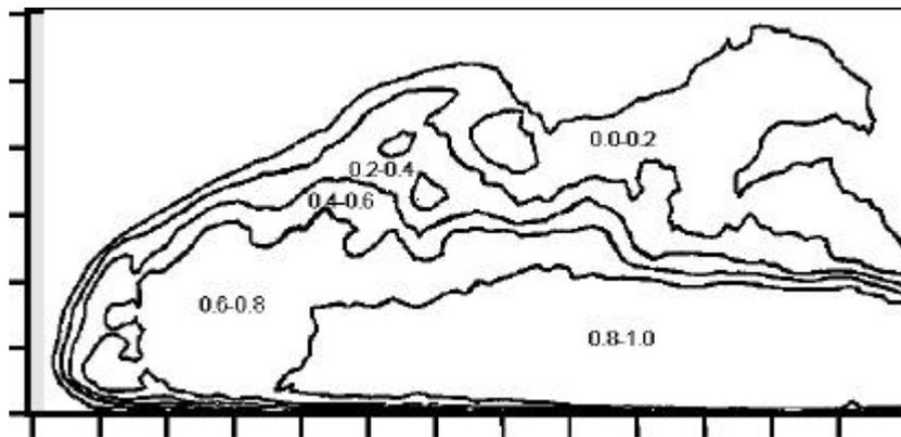
Fig. 5. Typical five-contour density profile map for the head of a gravity current flowing over a smooth surface with a 1% source fluid density excess. Scales shown are in 1 cm increments.
