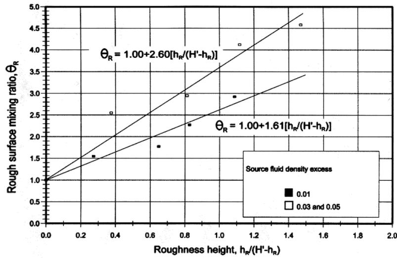
Fig. 8. Influence of the surface roughness scale on the rough-surface mixing ratio for flows with 1, 3 and 5% source fluid density excesses.
