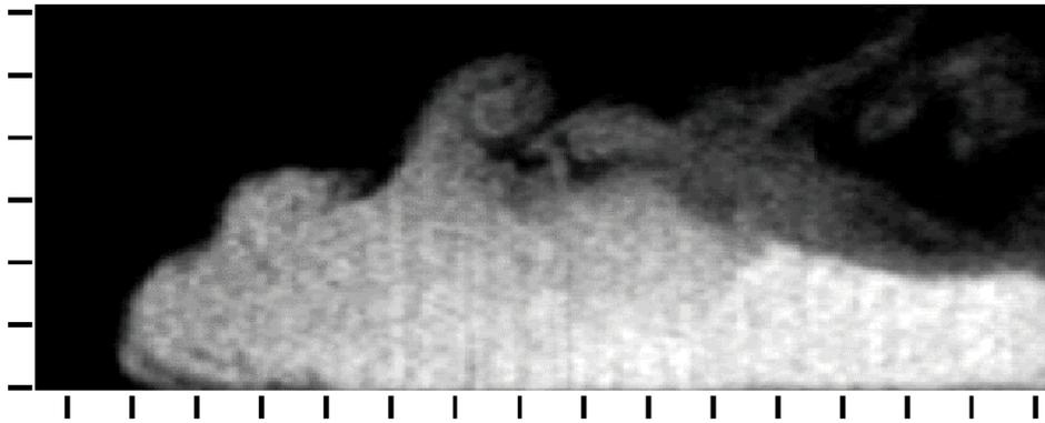
Fig. 2. Image of a typical gravity current head with a 1% source fluid density excess flowing to the left over a smooth surface. Scales shown are in 1 cm increments.
