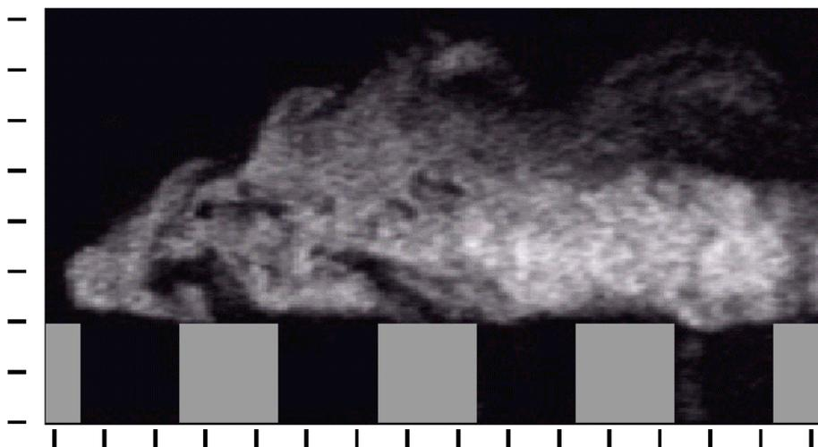
Fig. 1. Image showing internal mixing regions in a gravity current head with a 1% source fluid density excess flowing over a 19 mm roughness element array. Scales shown are in 1 cm increments.
