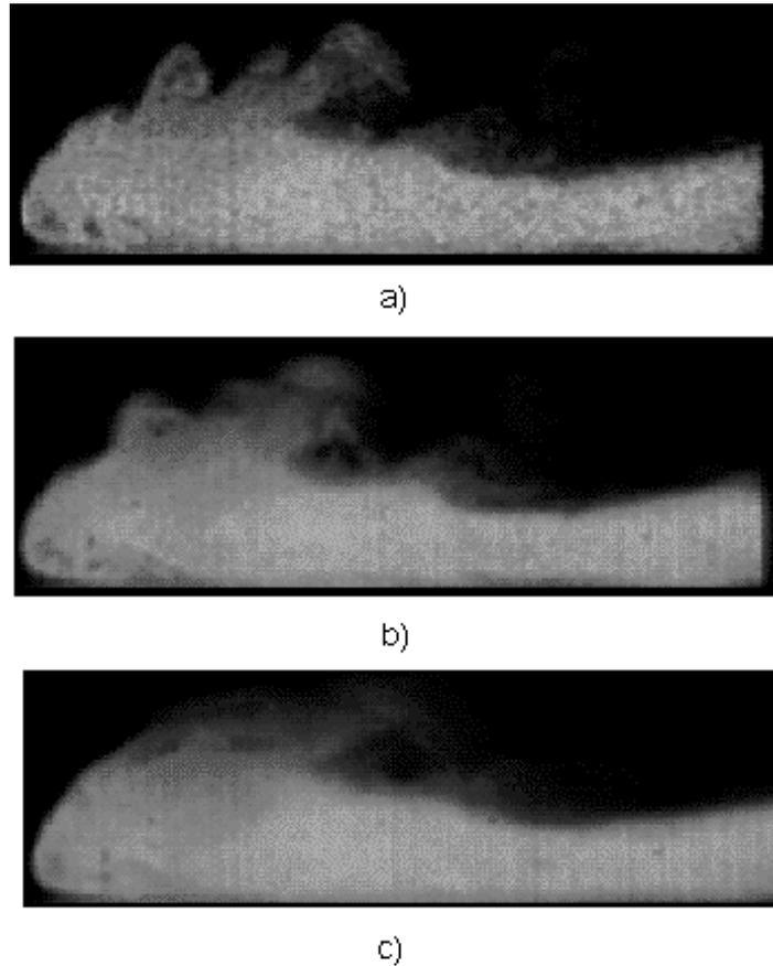
Fig. 6. Gravity current images that illustrate the effect of time averaging on the image detail for a) a single snapshot, b) a 10 frame average and c) a 30 frame average.
