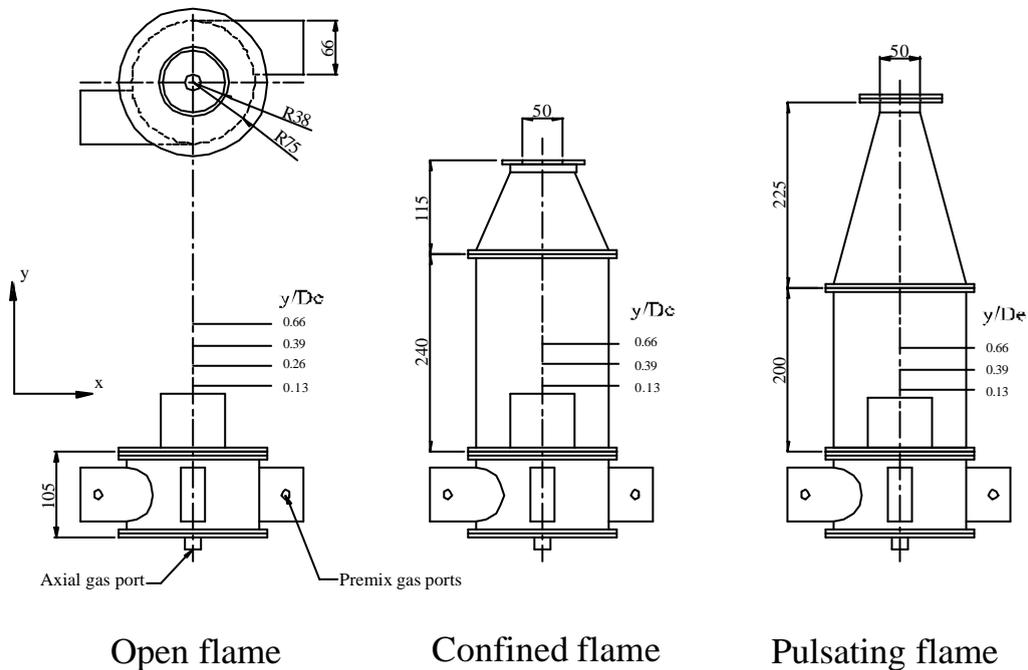
Figure 1 – Test rig schematic showing confinement geometries and LDA measurement positions
