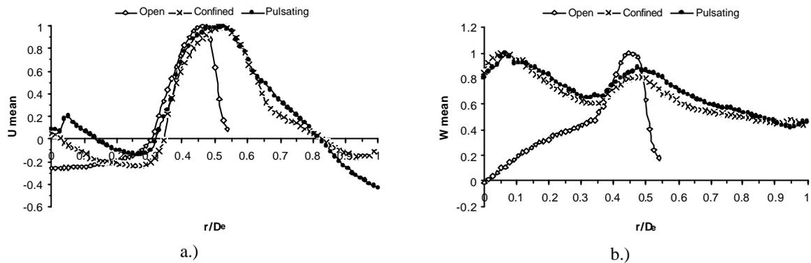
Figure 2 – Normalised mean a.) axial and b.) tangential velocities obtained under open, confined and resonant conditions
