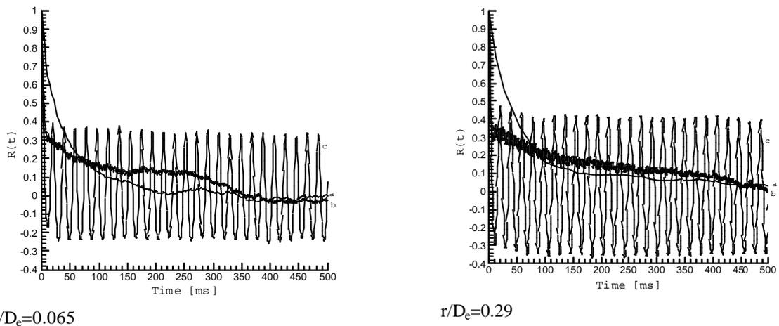
Figure 4. – Normalised time correlations for a) unconfined, b) confined and c) resonant conditions at  $L/D_e=0.13$
