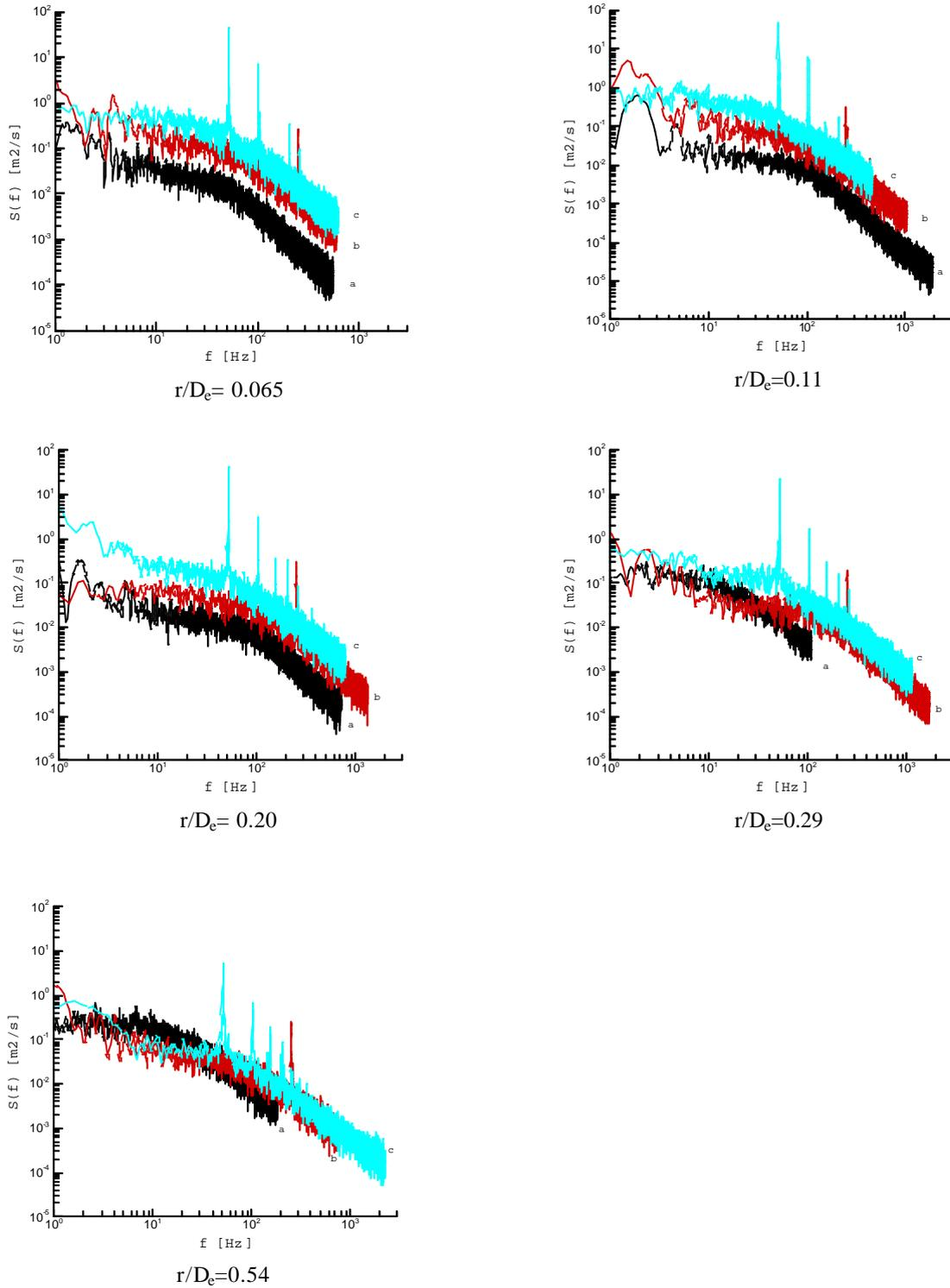
Figure 3. – Power Spectra for a) unconfined, b) confined and c) resonant conditions at  $x/D_c=0.13$
