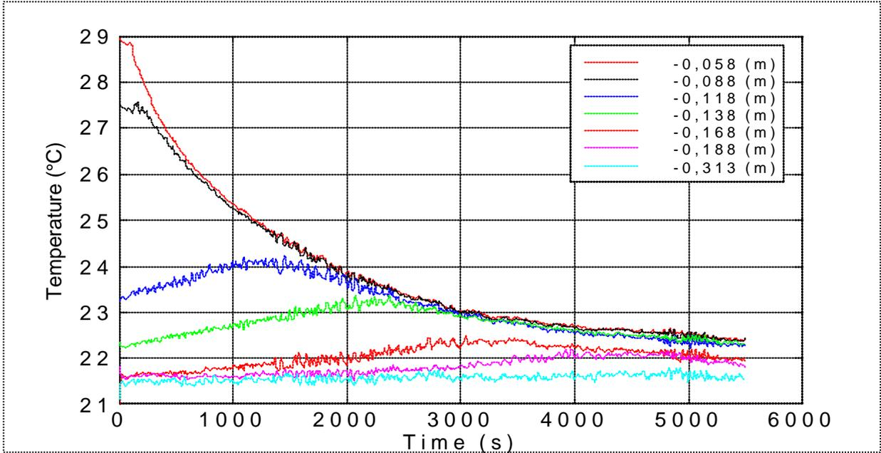
**Figure 9** Time series of temperatures measured by thermocouples at different depths
