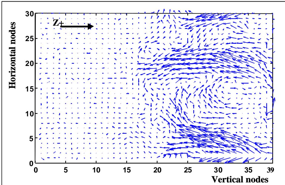
**Figure 13** Eulerian velocity field over a regular grid of 30 rows (horizontal) by 39 columns (vertical). Cell dimension is about 0.0065 m. ) Figure is rotated by 90° clockwise so that the free surface is on the right side)
