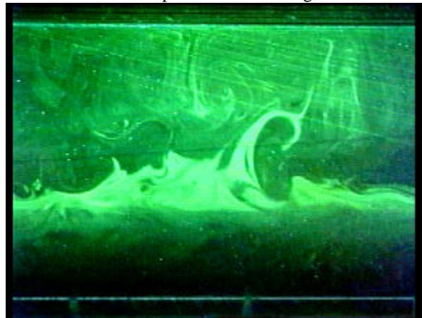
**Figure 2.** LIF visualization of the rise of heavier fluid inside the mixed layer
