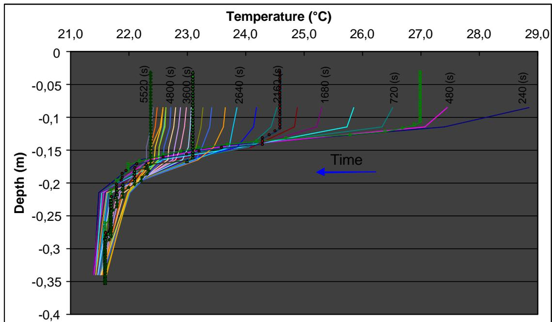
**Figure 8** Variation of Temperature at different depths versus time. The bold profiles are those measured by means of the mobile thermocouple.
