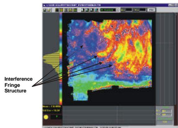
Fig. 9. An intensity flat field correction image containing interference fringes caused by the Iodine vapor cell windows.
