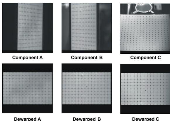
Fig. 12. Views of the image calibration target from the left, right, and above with an inclination angle of 30-degrees from the target plane before and after
