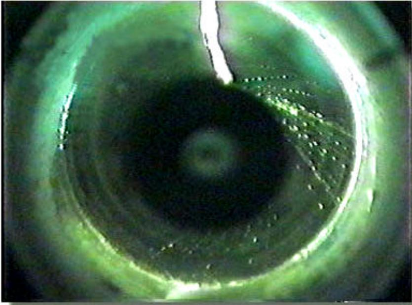
Figure 2: Typical flow visualisation image of the jet deflection.
