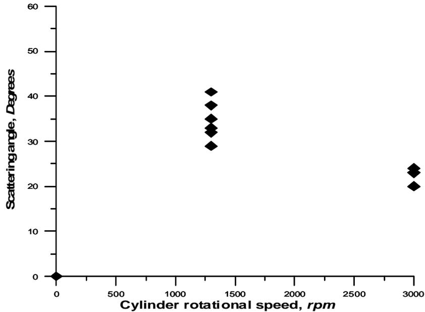
Figure 10: Scattering/expansion angle of the “secondary” jets versus the cylinder rotational speed
