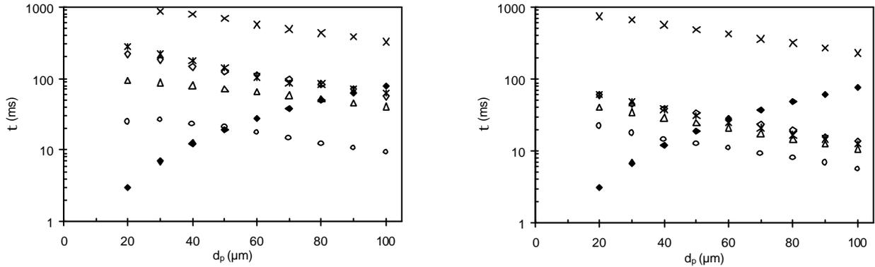
figure 6a (left) and 6b (right) : Comparison between the average time between collisions and the particle response time at different stations along the axis.
