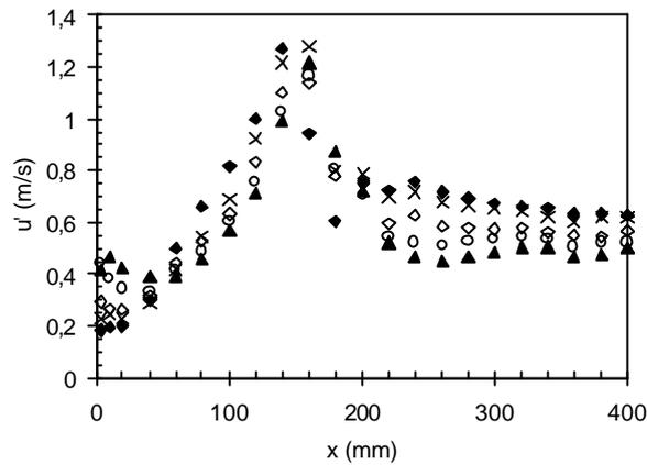
figure 3 : Axial evolution of the axial fluctuating velocity of continuous and dispersed phase at  $M_j = 22\%$  ? , Tracers ; **X**,  $d_p = 20\text{mm}$  ; ? ,  $d_p = 40\text{mm}$  ; ? ,  $d_p = 60\text{mm}$  ; ? ,  $d_p = 80\text{mm}$
