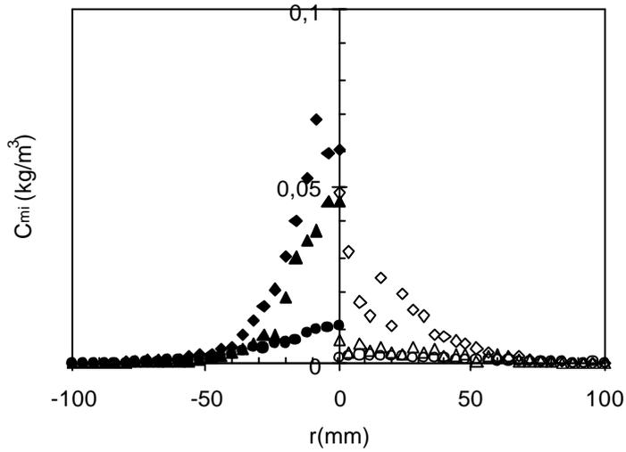
Figure 5 : Radial profiles of mean mass concentration  $C_{mi}$  (Right hand side and open symbols:  $M_j = 22\%$  ; Left hand side and dark symbols:  $M_j = 110\%$  and  $C_{mi}/5$  )
