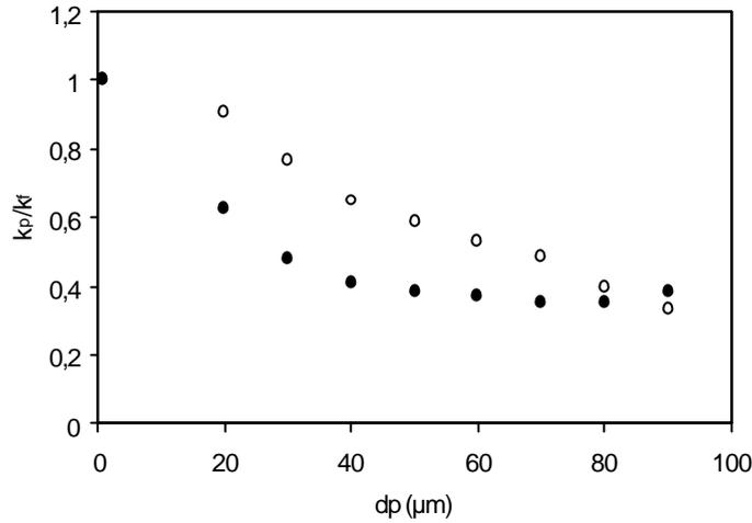
figure 7 : Evolution of the ratio of the turbulent kinetic energy  $k_p/k_f$  as a function of the size class on the axis at  $x = 240\text{mm}$ .  $?$ ,  $M_j = 22\%$  ;  $?$ ,  $M_j = 110\%$  .
