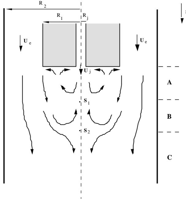
Figure 1 : Sketch of the confined bluff body flow in single phase configuration.
