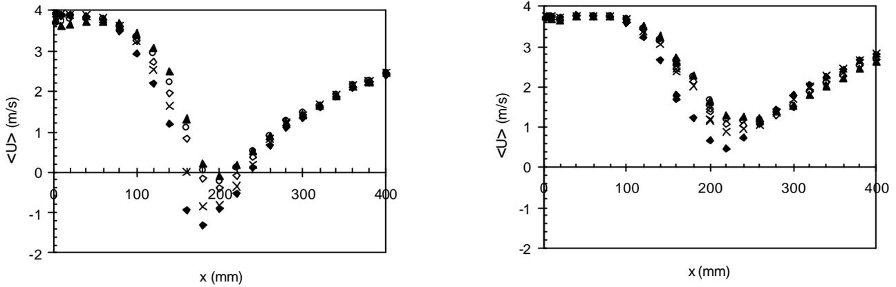
figure 2a (left) and 2b (right) : Axial evolution of the mean longitudinal velocity of continuous and dispersed phase at  $M_j = 22\%$  (left) and  $M_j = 110\%$  (right)
