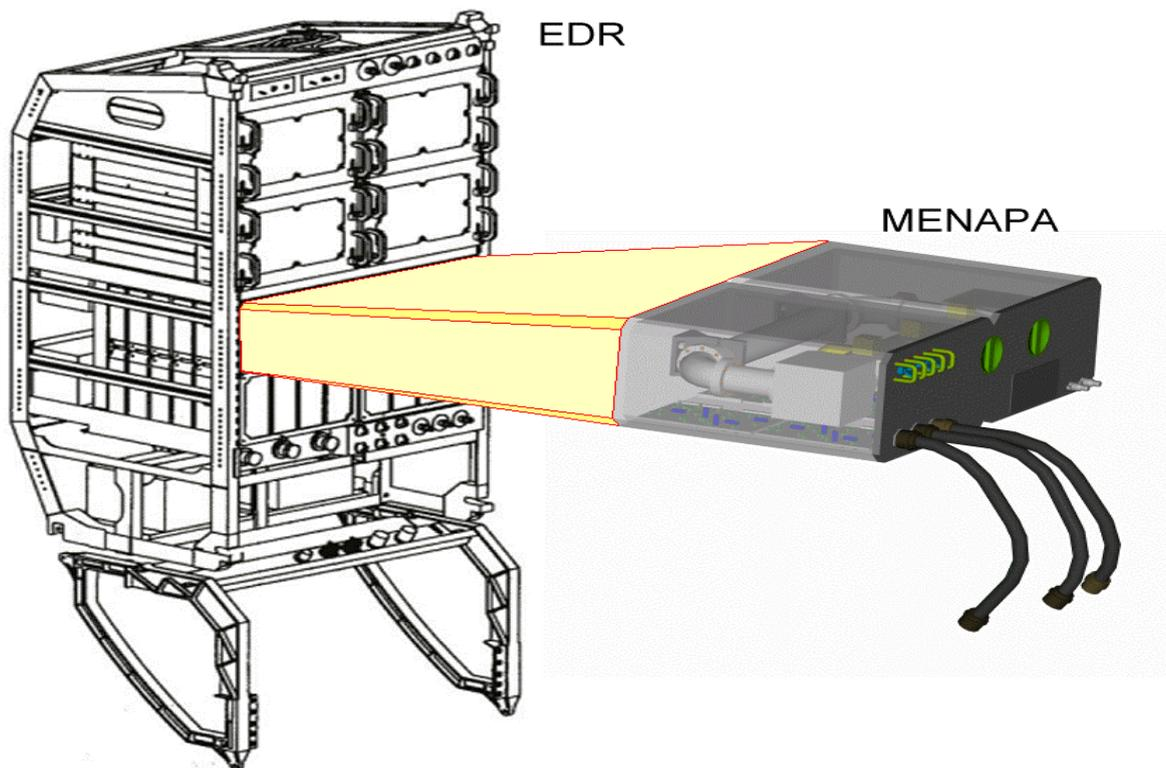
Figure 12: Integration of the modified tube reactor into the European Drawer Rack (EDR).
