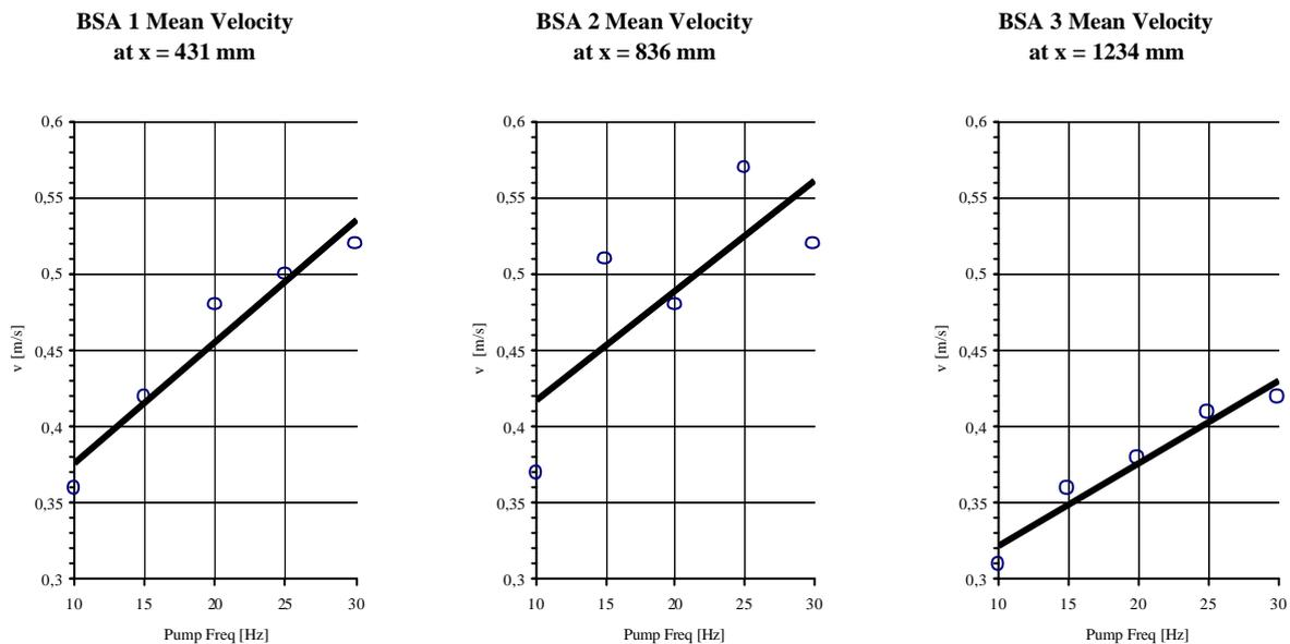
Figure 7: Flow rate in dependence on the power of the roots pump at a relative altitude of  $z = 55$ mm ( $y =$  middle of the tube).
