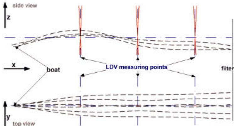
Figure 5: Principle sketch of the particle flow in relation to the LDV measuring plane.
