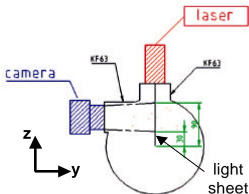
Figure 4: Sketch of the 90° visualisation arrangement (cross sectional view).
