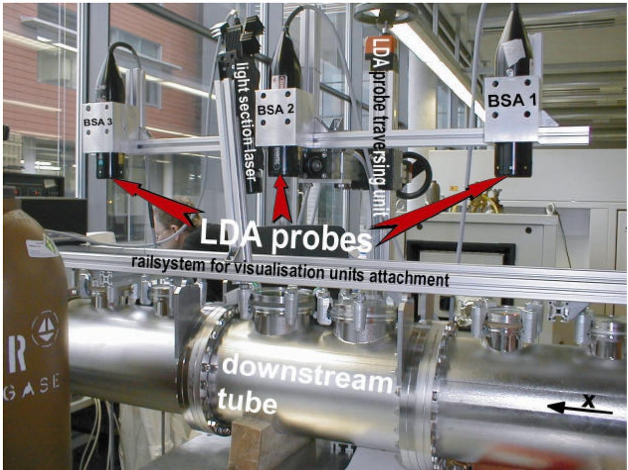
Figure 3: Photo of the LDV probe arrangement applied to the Inert Gas Condensation (IGC) process.
