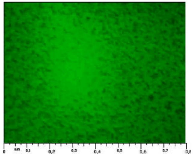
Figure 10: Snapshot of Particles between 2 and 10 µm on a glass substrate.
