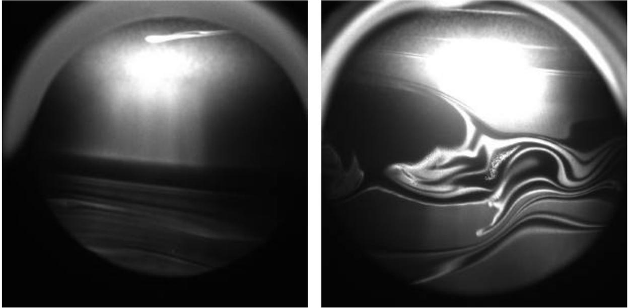
Table 3: PIV generated light sheet images taken at the second observation flange ( $x = 836$  mm), with the light sheet established at the horizontal centre line of the downstream tube (image dimensions:  $x = 132,6$  mm,  $z = 133,9$  mm). The used process parameters are listed in table 2.
