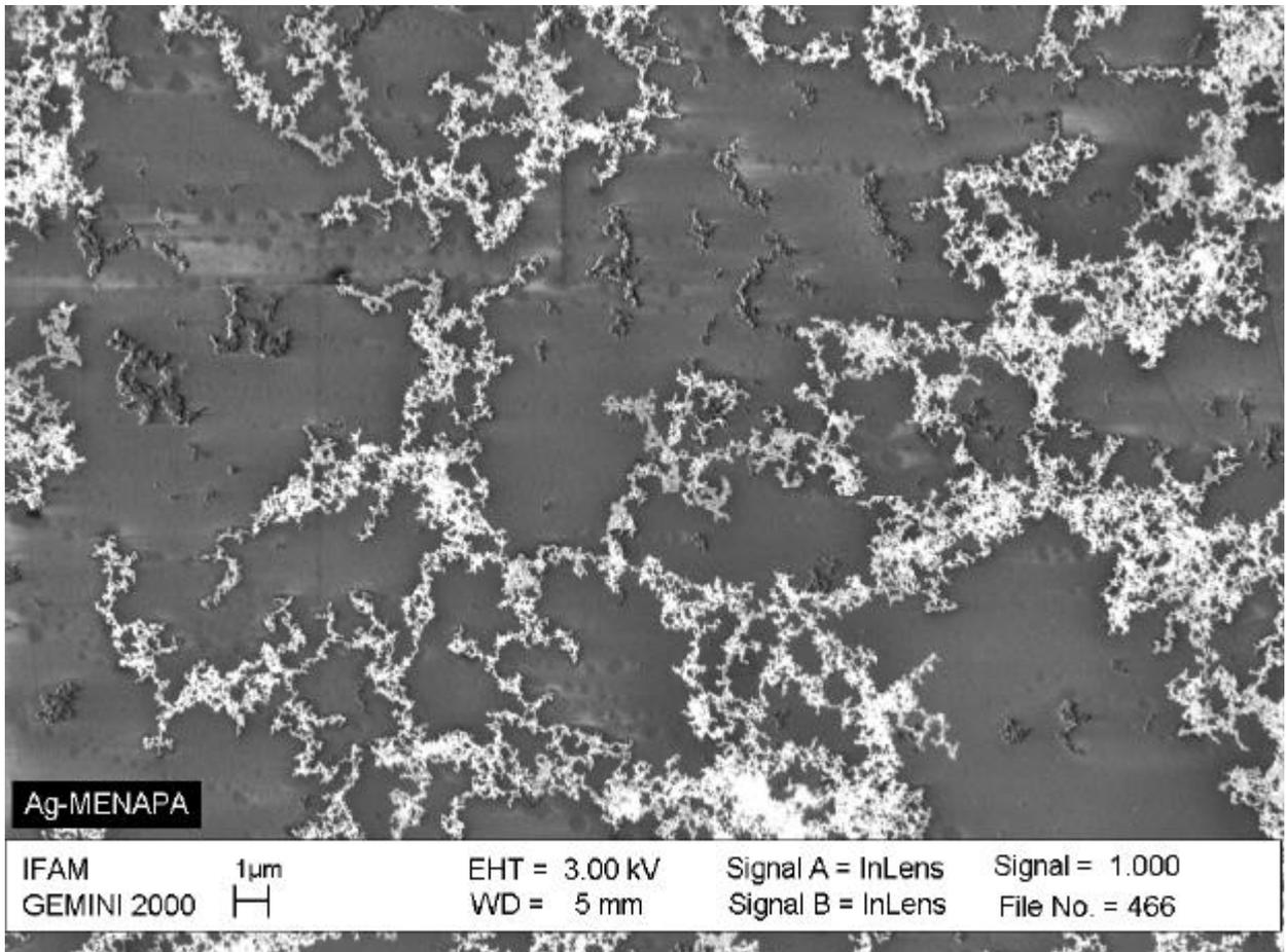
Figure 11: SEM picture of the particle layer on the glass substrate.
