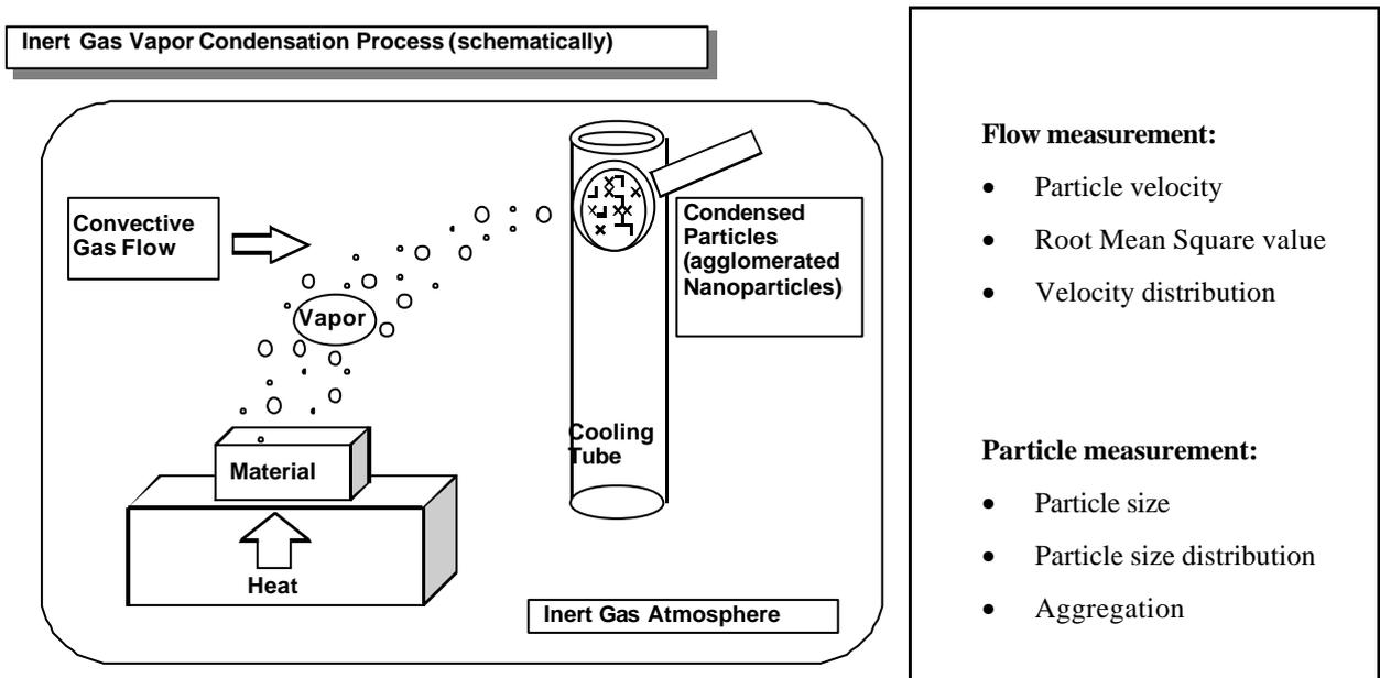
Figure 1: Principle sketch of the Inert Gas Condensation Process (IGC).
