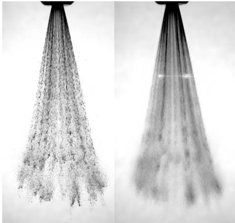
Figure 1 Single Fluid GDI Spray with Wide Poly-disperse Drop Size Distribution
