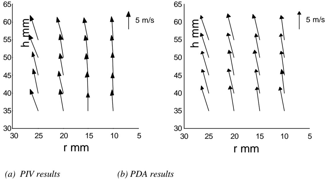
Fig. 5 Comparison of mean velocity vectors measured by PIV and PDA experiments
