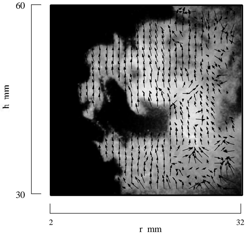
*Fig. 4 Instantaneous velocity field measured by the PIV system.
