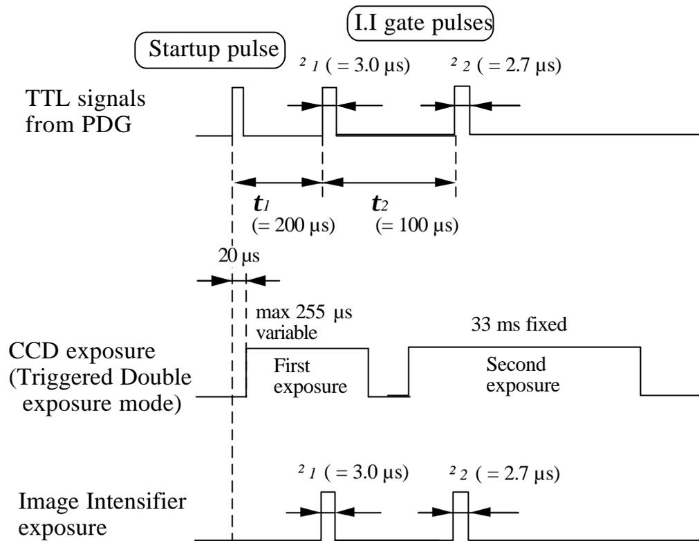
Fig. 3 Pulse and exposure time chart for PIV measurement
