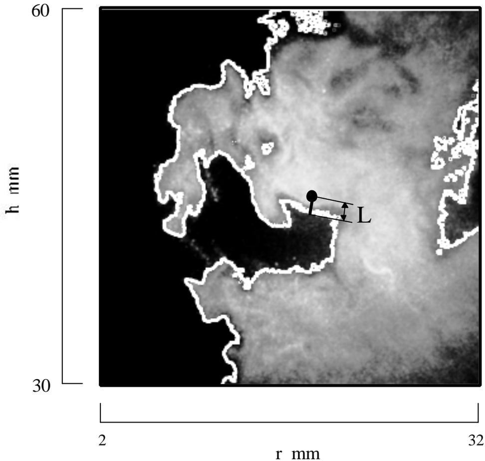
*Fig. 6 The contours of the spray boundary obtained by binarizing the spray image. A closed circle indicates the measurement location of MICRO probe system.*
