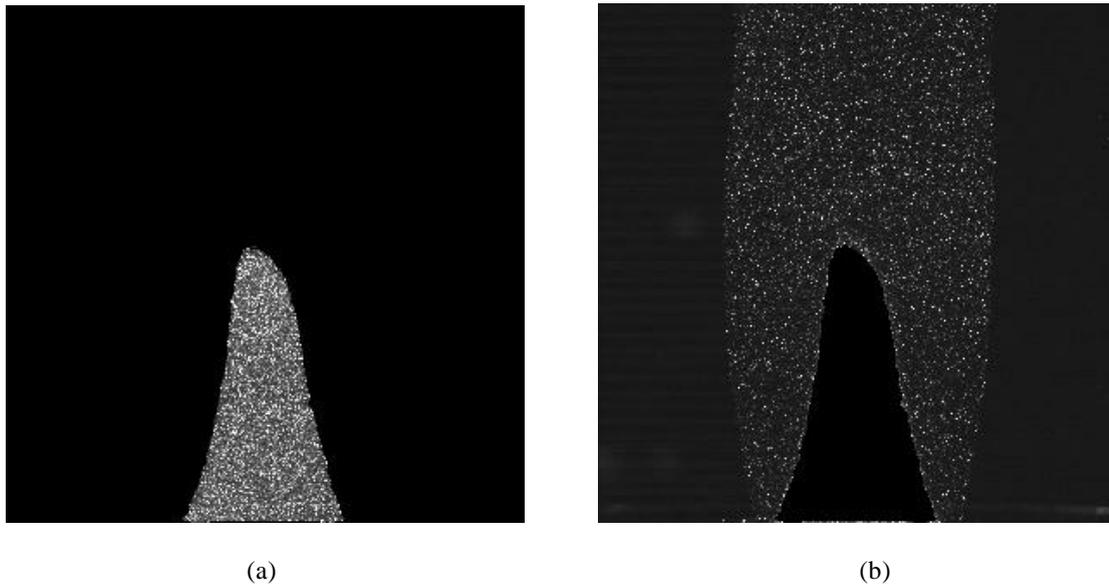
*Fig. 8. Separation of the PIV images
