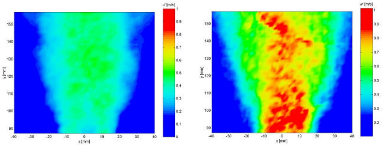
Fig. 8 Turbulent fluctuations at the center plane.
