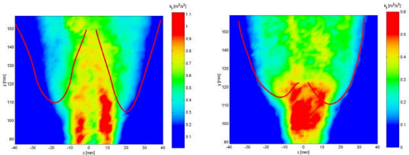
Fig. 9 Turbulent kinetic energy distribution.
