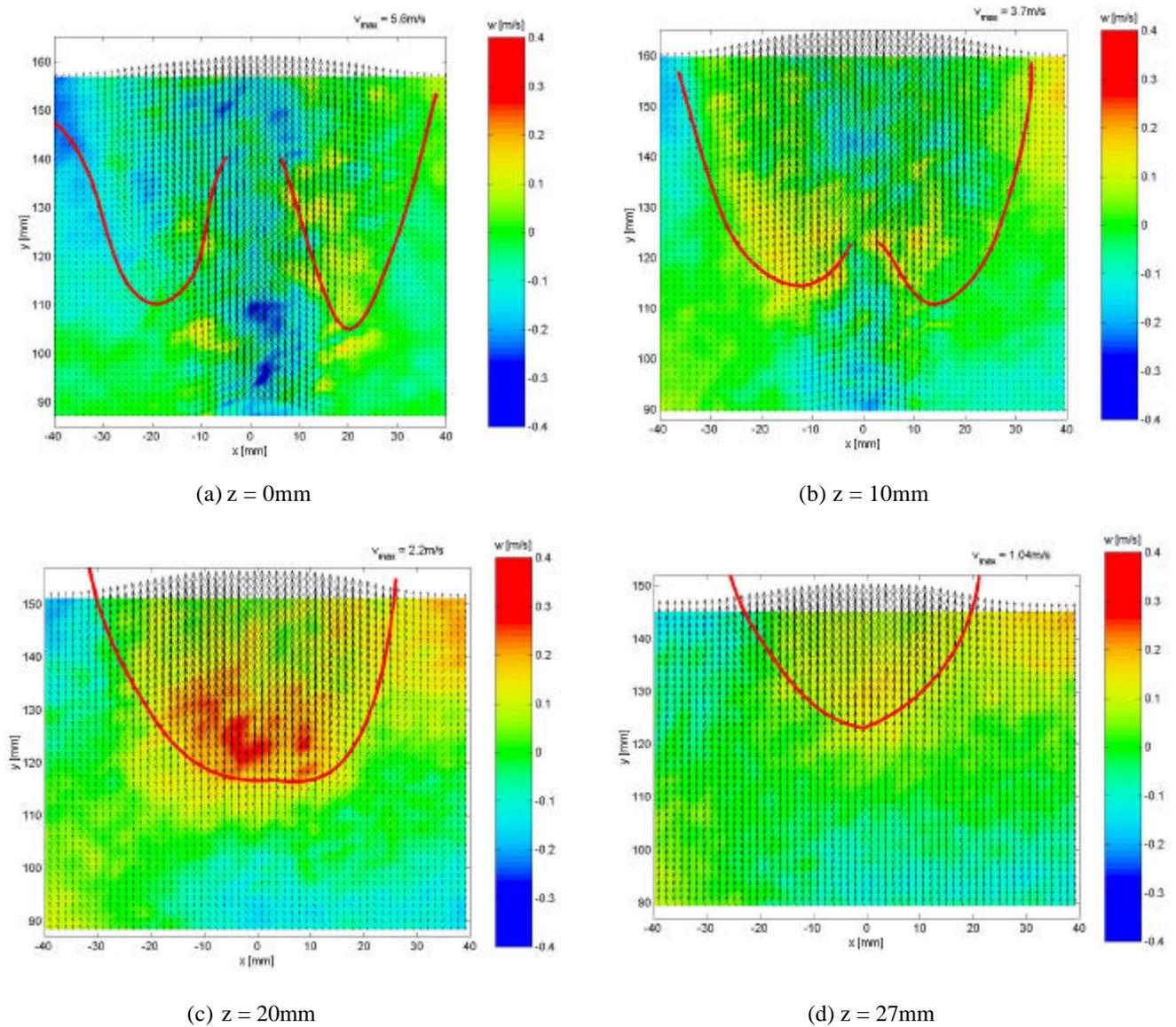
Fig. 6 Averaged velocity fields at the flame base of a lifted flame.
