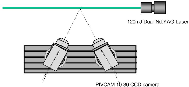
Fig. 2 Two-Camera Scheimpflug arrangement for stereoscopic PIV measurements.
