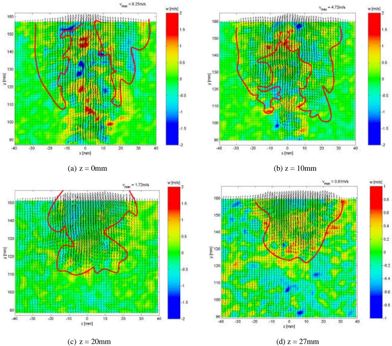
Fig. 5 Instantaneous velocity fields at the flame base of a lifted flame.
