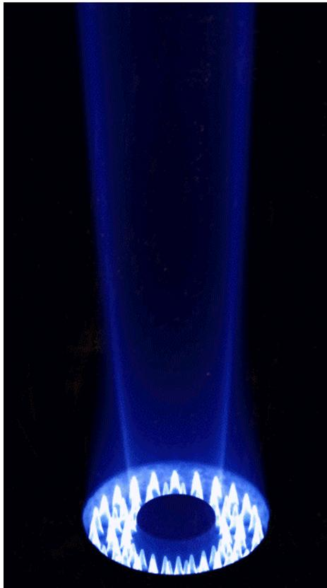
Figure 3. Piloted diffusion flame burner (Barlow and Frank, 1998a).
