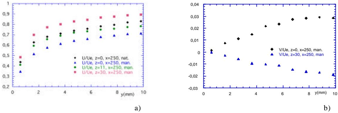
Fig. 4. Mean longitudinal (a) and wall normal (b) velocity profiles, at  $x=250\text{mm}$ .
