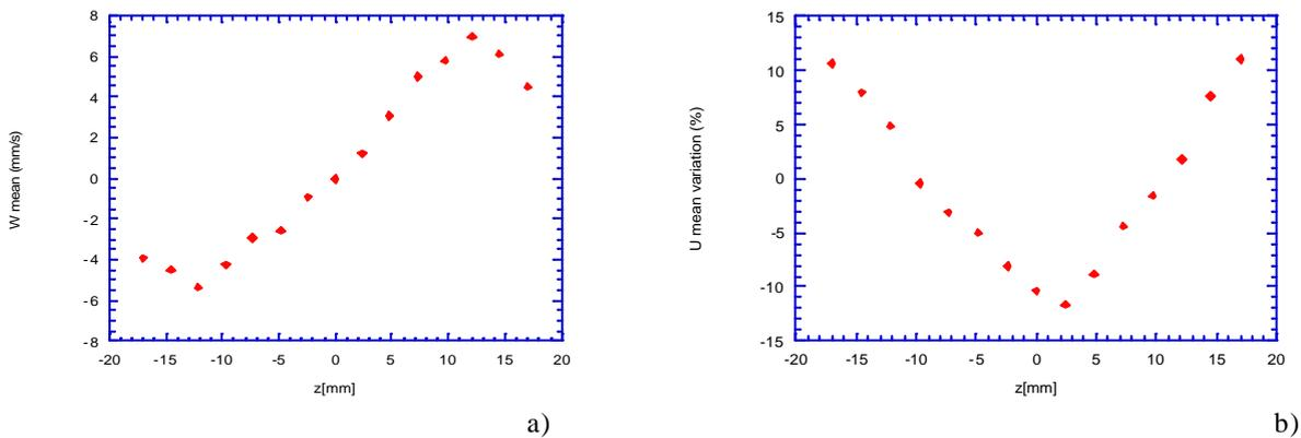
Fig. 5. Mean spanwise velocity  $W$ -distribution (a) and percent variation of mean longitudinal velocity  $U$ -distribution (b) at  $x=250\text{mm}$  and  $y^+ > 20$ .
