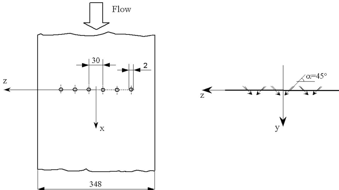
Fig. 1. Sketch of the flat plate with jet holes configuration and reference system. Dimensions in millimeters.
