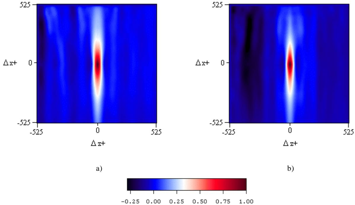
Fig. 6. Double spatial correlation  $R_{uu}$ , at  $y^+ \gg 20$ , in the natural case (a) and manipulated case (b).
