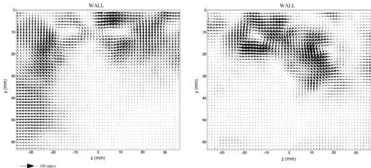
Fig. 2. Instantaneous vectorial velocity fields in the (y,z) plane at  $x=130\text{mm}$ .
