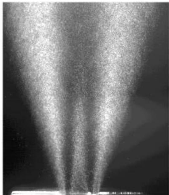
**Fig 9a: Instantaneous Tomographic image of H2/O2 Non-premixed flame, with ZrO<sub>2</sub> seeding (1mm=11pix)**
