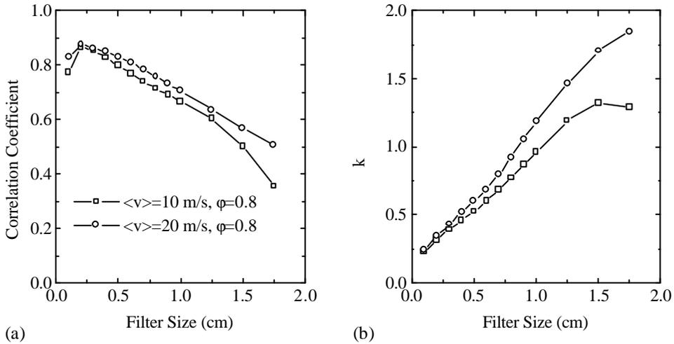
Figure 9. The influence of the filter size on the correlation between the unresolved flame surface density and the proposed model (a) and on the model parameter  $k$  (b).
