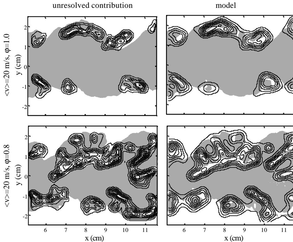
Figure 10. Iso-contours of the unresolved flame surface density (on the left) and the proposed model (on the right) with  $D=5$  mm and  $k=0.6$  for two different operating conditions. In gray is shown the binarized progress variable. Units are in cm.
