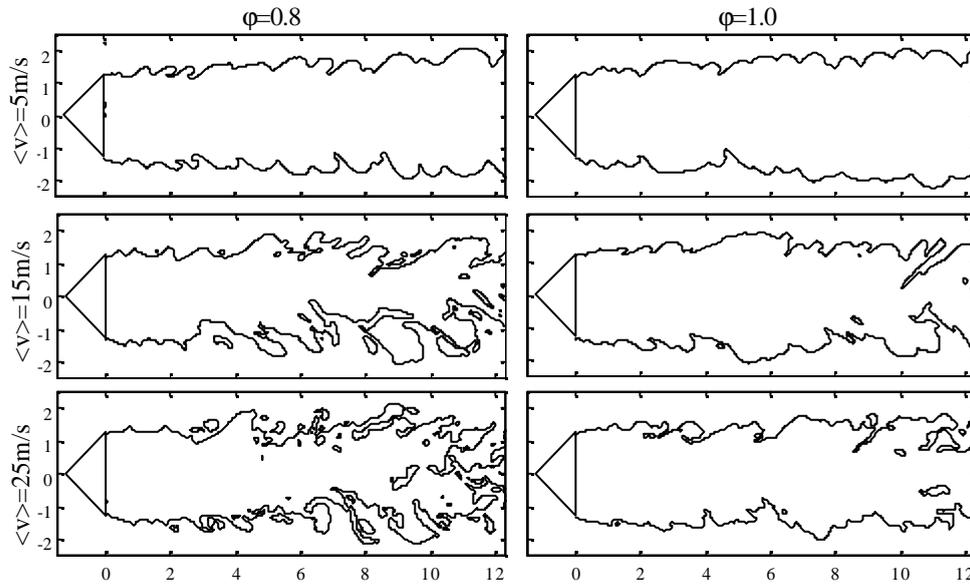
Figure 4. Instantaneous flame fronts extracted from OH-LIF images at various operating conditions. Mean velocity and equivalence ratio of the propane/air mixture at the inlet are indicated.
