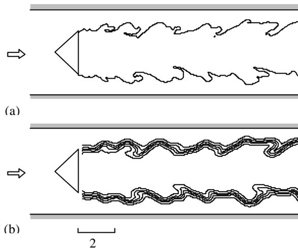
Figure 1. Visualization of the instantaneous flame front of a premixed turbulent propane/air flame stabilized behind a triangular flame holder (a) (mean inlet velocity  $\langle v \rangle = 10 \text{ m/s}$ , equivalence ratio  $j = 0.8$ ) and
