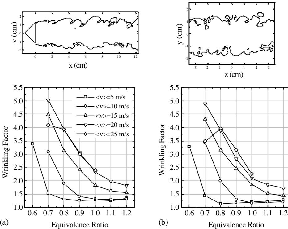
Figure 6. Flame surface wrinkling factor calculated from the downstream images (a) and the transverse images (b) at  $x = 8$  cm from the flame holder for various operating conditions. Results are calculated from areas indicated in the upper images.
