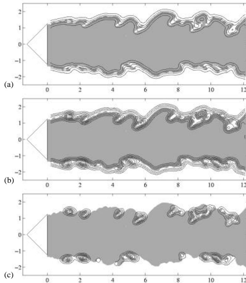
Figure 7. The filtered progress variable  $\bar{c}$  (a), the flame surface density  $\mathbf{S}$  (b) and the unresolved contribution  $\Sigma - |\nabla \bar{c}|$  (c). In gray is displayed the binarised progress variable  $c$ .
