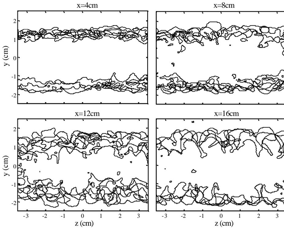
Figure 5. Instantaneous flame fronts in the plane perpendicular to the downstream direction at 4, 8, 12 and 16 cm from the flame holder for  $\langle v \rangle = 20$  m/s and  $j = 1.0$  (conditions corresponding to figure 3). Each figure contains four realizations.
