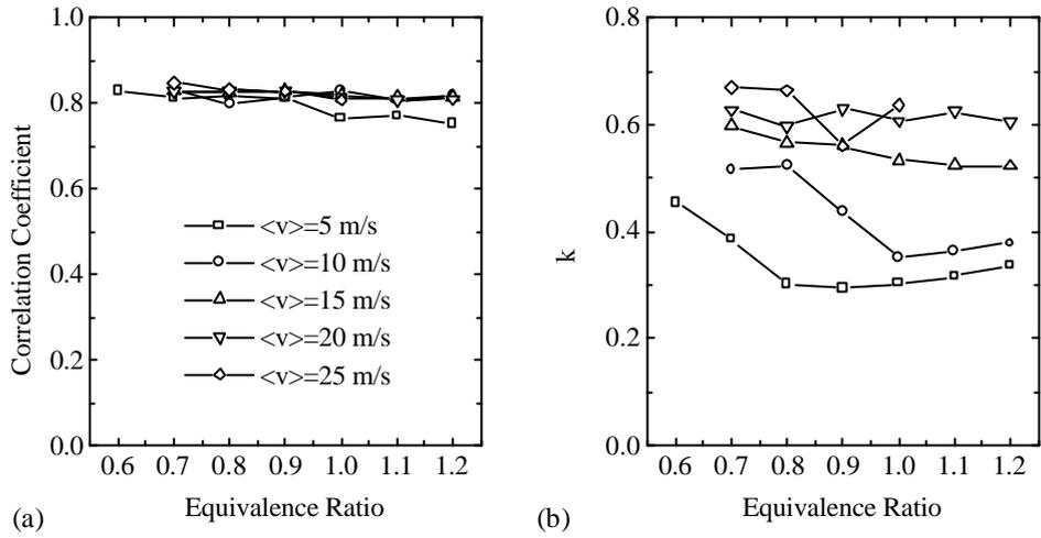
Figure 8. The correlation between the unresolved flame surface density and the proposed model (a) and the estimation of the model parameter  $k$  using the least-squares method (b).
