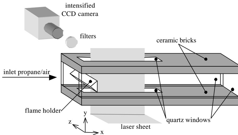
Figure 2. Experimental configuration. A propane/air mixture is injected into the combustion chamber and a turbulent flame is stabilized behind a triangular-shaped obstacle. LIF images are obtained by passing a laser sheet through two narrow windows and visualizing the resulting radiation with an intensified CCD camera.
