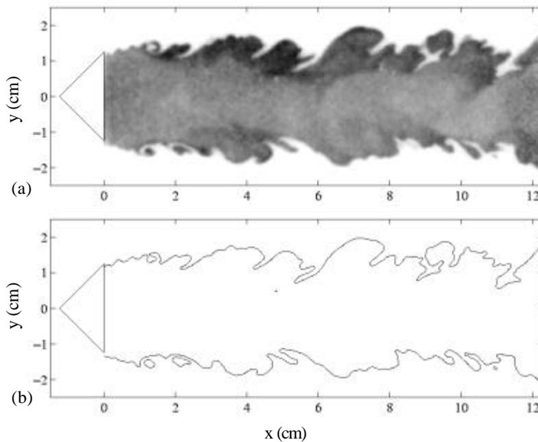
Figure 3. Instantaneous LIF image of the OH radical in a turbulent premixed propane/air flame stabilized on a triangular-shaped obstacle ( $\langle v \rangle = 20$  m/s and  $j = 1.0$ ) (a) and the extracted flame front (b).
