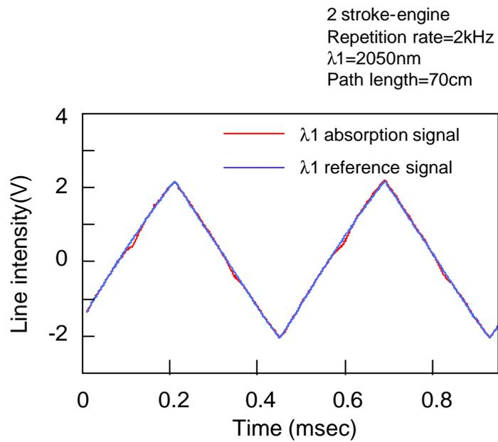
Fig. 12 Direct absorption measurement in exhaust pipe gas of 2 stroke engine
