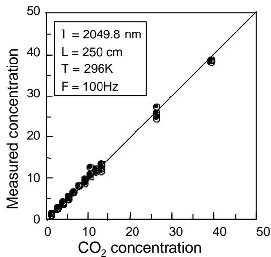
Fig.9 Comparison of measured CO<sub>2</sub> concentration to absolute value
