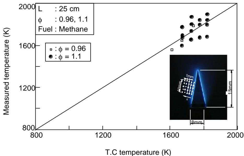
Fig.10 Comparison of temperature measured in the CH<sub>4</sub> + air flame Determined from 2-color method and type-R thermocouple
