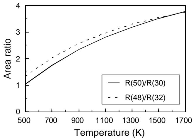
Fig. 5 Temperature dependence of the integrated intensity ratio
