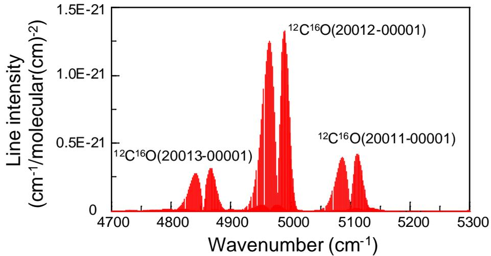
Fig. 4 CO<sub>2</sub> absorption line near 2000nm at 296K(HITRAN96,98)
