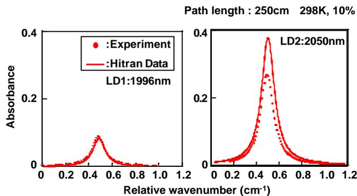
Fig. 7 Direct absorption measurement using developed two DFB laser
