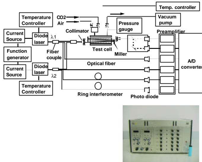
Fig. 6 Schematic layout of developed sensor system
