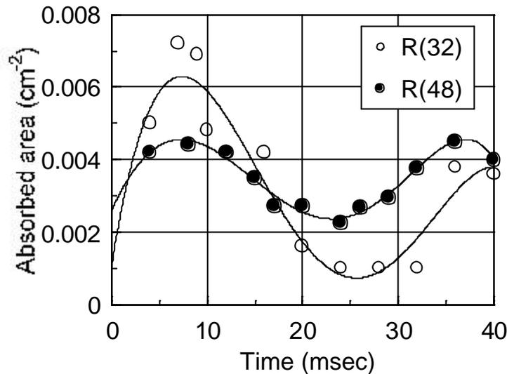
Fig. 13 Absorbed area change in exhaust pipe gas of 2 stroke engine
