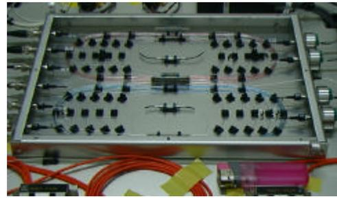
*Developed fiber ring interferometer*
