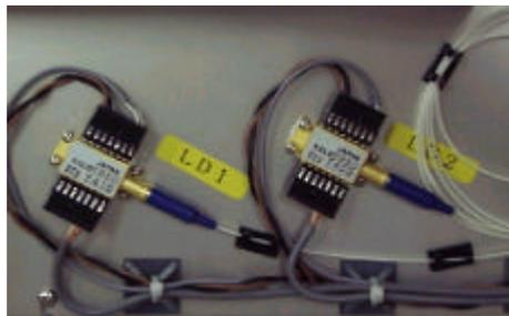
Fig. 1 Pigtail DFB laser module
