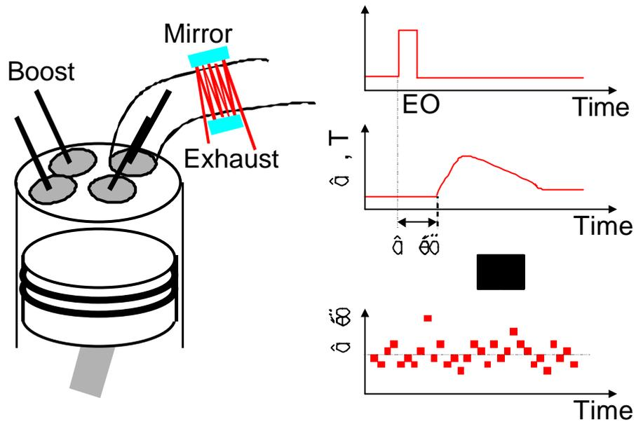
Fig. 11 Gas temperature and hot gas arrival time
