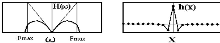
Fig.6 Shepp and Rogan's filter function<sup>[26]</sup>.
