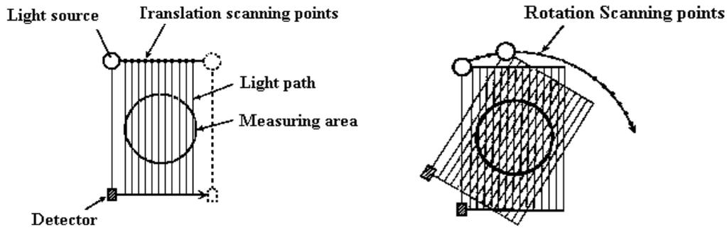
Fig.4 Translation-rotation (T-R) scanning for computer tomography.
