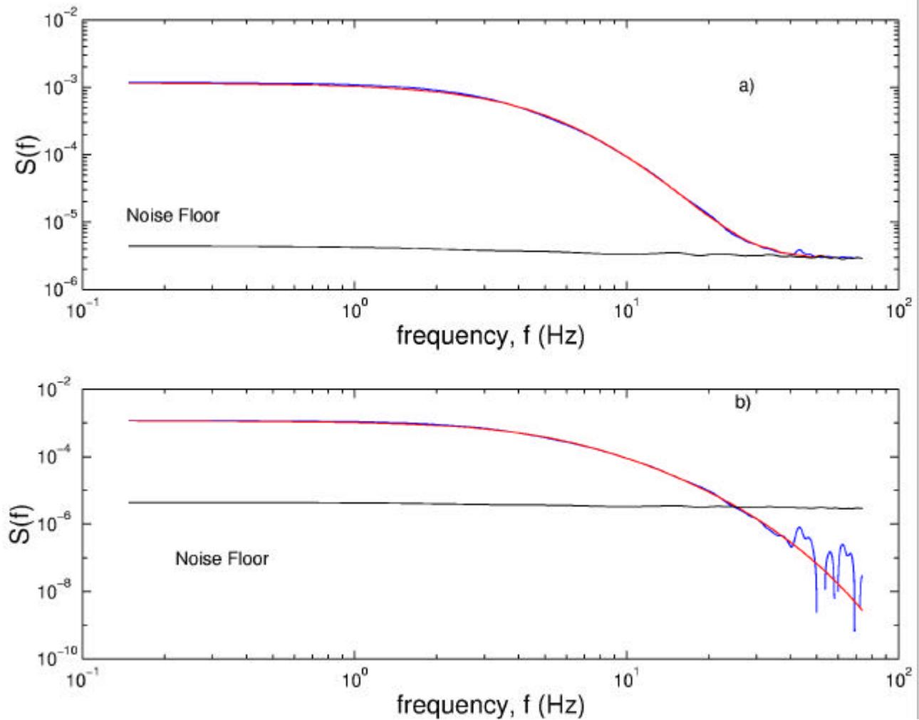
Figure 6: Comparison between the variance spectrum ( $m^2/s^2\text{-Hz}$ ) of the observations (blue line) and the algebraic-exponential two-scale model (red line). In b) the noise component  $G(f)$  has been subtracted from model and observations.
