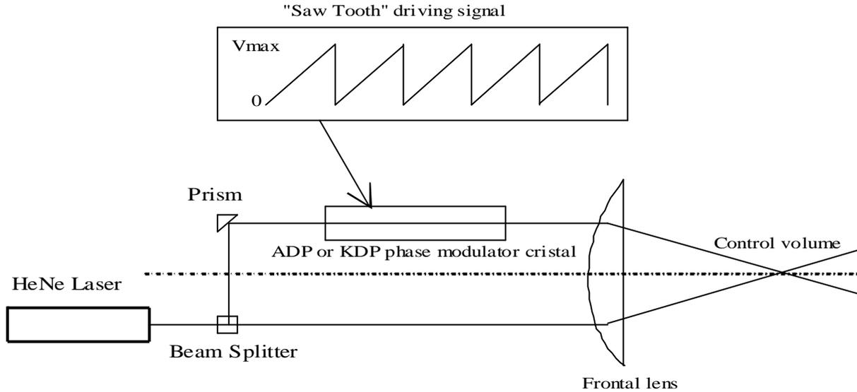
Figure 1: Schematic layout of the new LDV system
