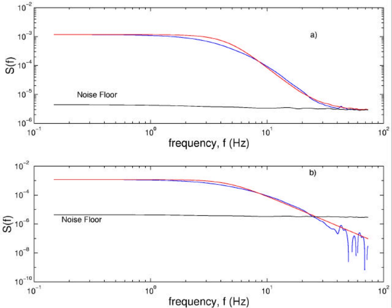
Figure 4: Comparison between the variance spectrum ( $m^2/s^2$ -Hz) of the observations (blue line) and the power law (algebraic) model (red line). In b) the noise component  $G(f)$  has been subtracted from model and observations.
