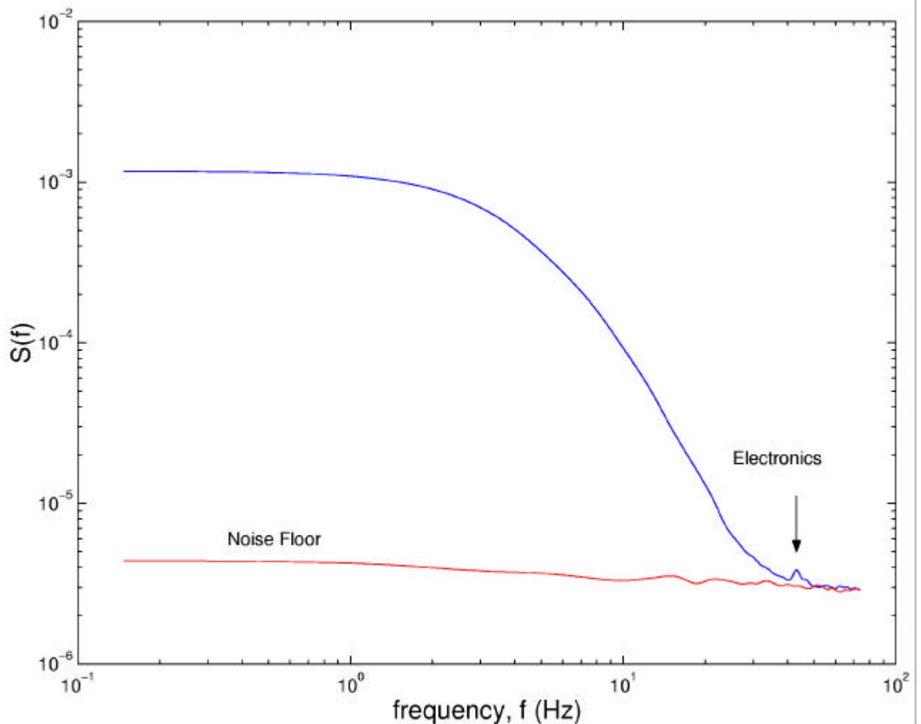
Figure 2: Variance spectrum ( $m^2/s^2$ -Hz) against the frequency for the velocity series  $V(iDt)$  for  $Re=5000$ . The red lines is the power spectrum of the LDV noise affecting the velocity series.
