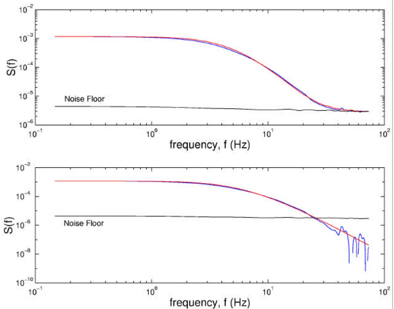
Figure 5: Comparison between the variance spectrum ( $m^2/s^2$ -Hz) of the observations (blue line) and the two-scale algebraic model (red line). In b) the noise component  $G(f)$  has been subtracted from model and observations.
