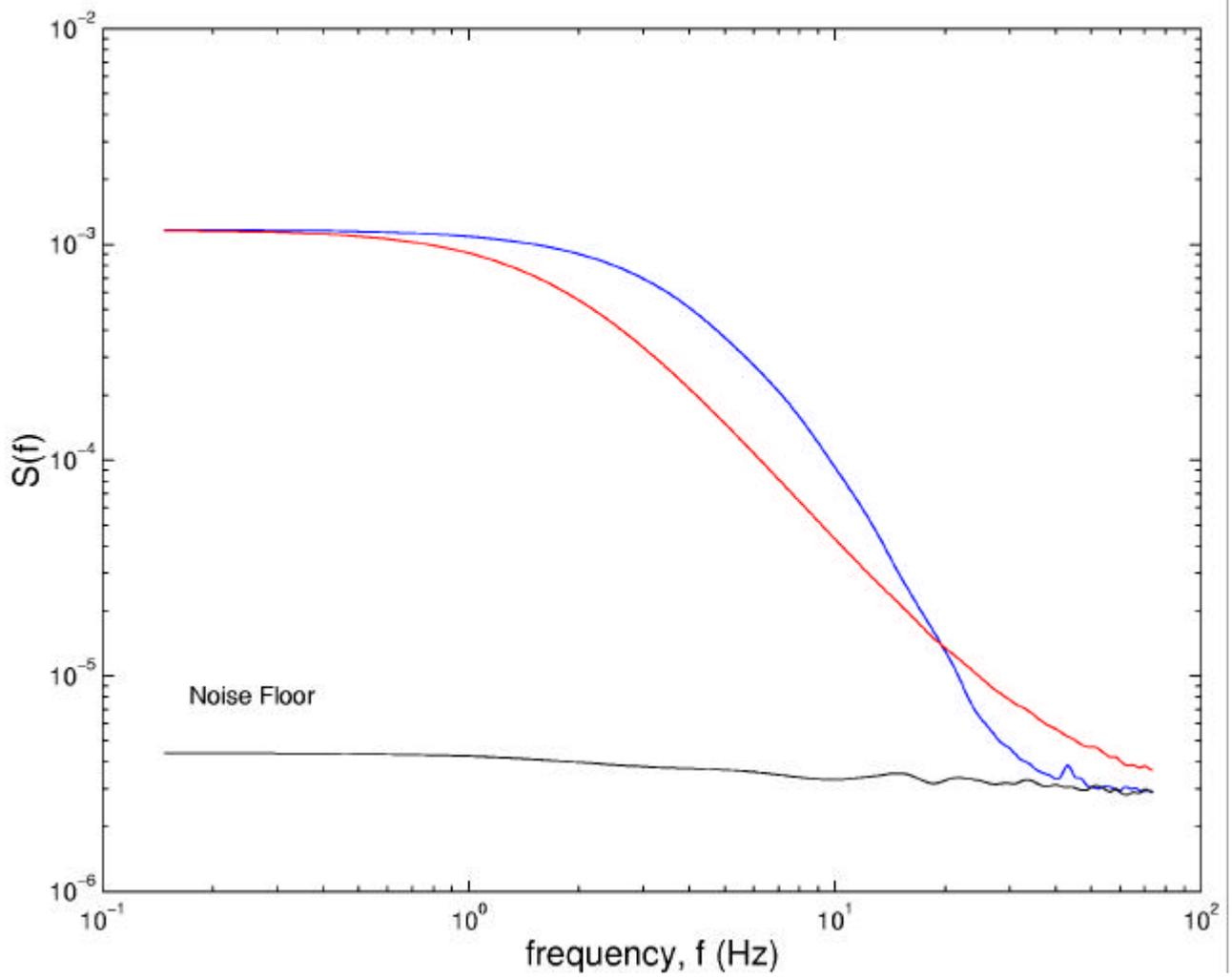
Figure 3: Comparison between the variance spectrum ( $m^2/s^2$ -Hz) of the observations (blue line) and the Lorentzian-shape model (red line).
