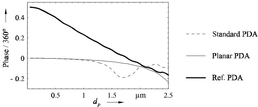
Fig. 6: Phase difference as a function of the particle diameter for a standard PDA ( $\varphi=30^\circ$ ,  $\psi=\pm 20^\circ$ ), planar PDA ( $\varphi=0^\circ$ ,  $\psi=\pm 20^\circ$ ) and reference beam PDA ( $m=1.33$ ,  $\lambda=852$  nm,  $\theta=9^\circ$ )
