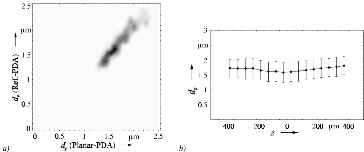
Fig. 10: Coincident measurements with planar and reference beam PDA: a) correlation of measured particle sizes, b) measured particle sizes as a function of the z-coordinate inside the measurement volume of the planar PDA ( $m = 1.33$ ,  $\lambda = 852\ \text{nm}$ ,  $\theta = 9^\circ$ , Planar-PDA:  $\psi = \pm 11.5^\circ$ )
