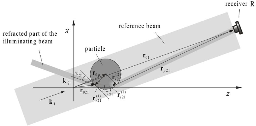
Fig. 4: Signal generation for the reference beam technique by refraction
