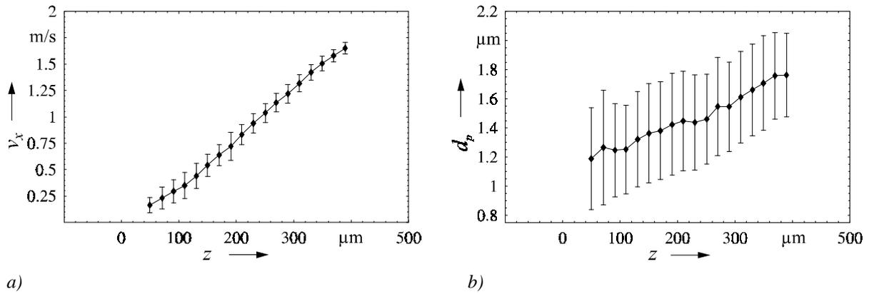
Fig. 11: Local dependencies of the velocity (a) and detected particle sizes (b) in a boundary layer of a plane plate in a free flow of a seeding generator measured with the reference beam PDA ( $z$ -coordinate perpendicular to the surface of the plate with respect to the center of the measurement volume)
