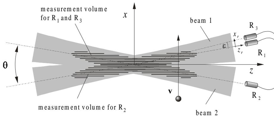
Fig. 1: Beam and receiver alignment of a reference beam PDA
