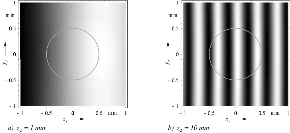
Fig. 2: Interference of the reference beam with the scattered wave in the plane of receiver  $R_1$  for two different positions of the scattering particle along the beam axis of the illuminating beam  $z_2$  (calculated by light scattering analysis according to the Fourier-Lorenz-Mie theory (FLMT, Albrecht et al. 1995), Parameters:  $\lambda = 852 \text{ nm}$ ,  $\theta = 9^\circ$ ,  $r_{01} = 0.7 \text{ m}$ , radius of the beam waist  $r_b = 65 \mu\text{m}$ )
