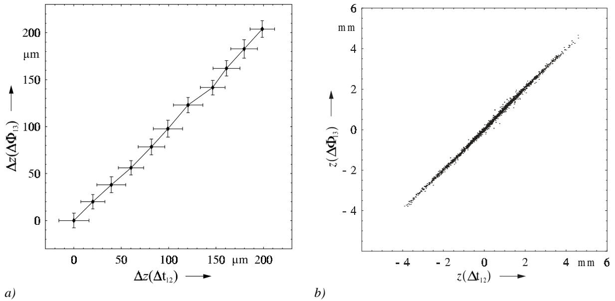
Fig. 9: a) Comparison between time displacement and phase difference method for a location of the position of a wire (diameter  $25\ \mu\text{m}$ ) in the measurement volume, b) correlation of coincident measurements with both systems in front of a wind tunnel nozzle
