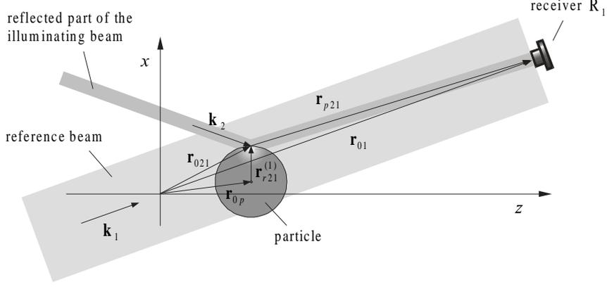
Fig. 3: Signal generation for the reference beam technique by reflection
