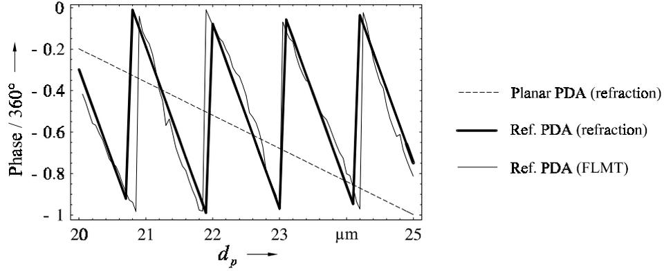
Fig. 5: Phase difference for refraction as a function of the particle diameter for a planar and reference beam PDA (Parameters:  $m=1.33$ ,  $\lambda=852$  nm,  $\theta=18.9^\circ$ , Planar PDA:  $\psi=\pm 13^\circ$ )
