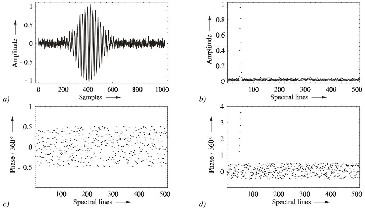
Fig. 8: a) Alternating part of the received Doppler signal, b) Amplitude spectrum, c) Phase spectrum, d) Phase spectrum with eliminated  $2\pi$  ambiguities
