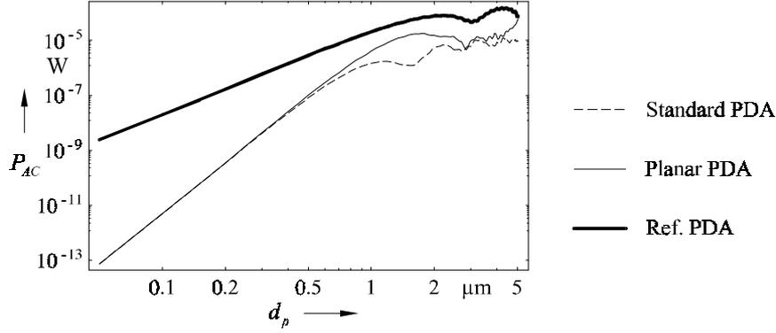
Fig. 7: Alternating part of the light power on the receiver as a function of the particle diameter (Parameters:  $m = 1.33$ ,  $\lambda = 852$  nm,  $\theta = 9^\circ$ ) for a standard PDA ( $\varphi = 30^\circ$ ,  $\psi = \pm 20^\circ$ ,  $NA = 0.05$ ), planar PDA ( $\varphi = 0^\circ$ ,  $\psi = \pm 20^\circ$ ,  $NA = 0.05$ ) and reference beam PDA ( $NA = 7.1 \times 10^{-4}$ )
