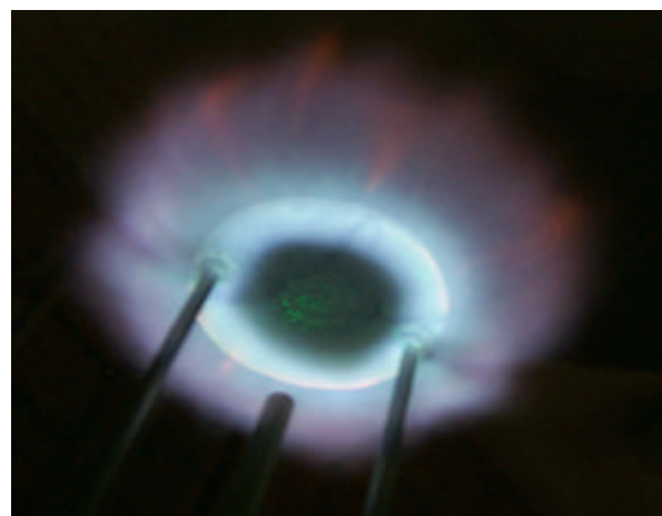
Fig. 4: View on the stagnation plate with the flame
