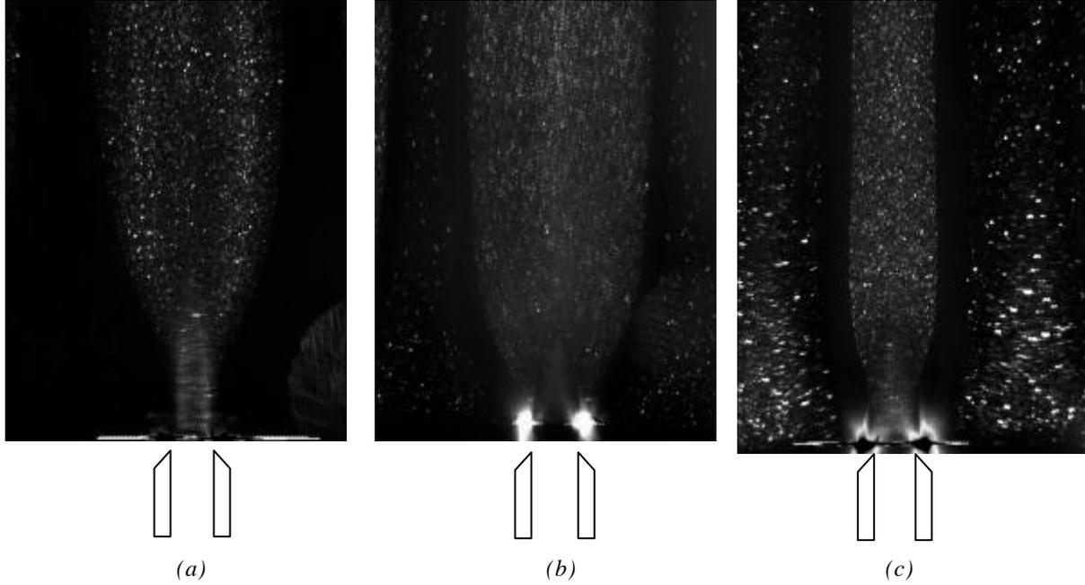
Figure 4: Particle images obtained above one burner slot for flame condition #1, 2 and 3, from left to right.
