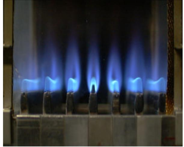
Figure 2: Photograph of the multiple slot burner.
