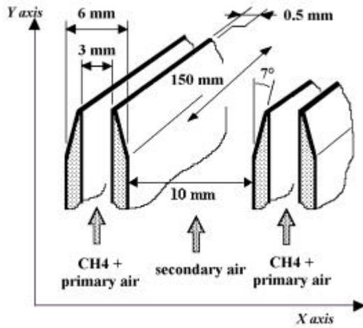
Figure 1: Schematic of two of the seven rectangular burner slots.
