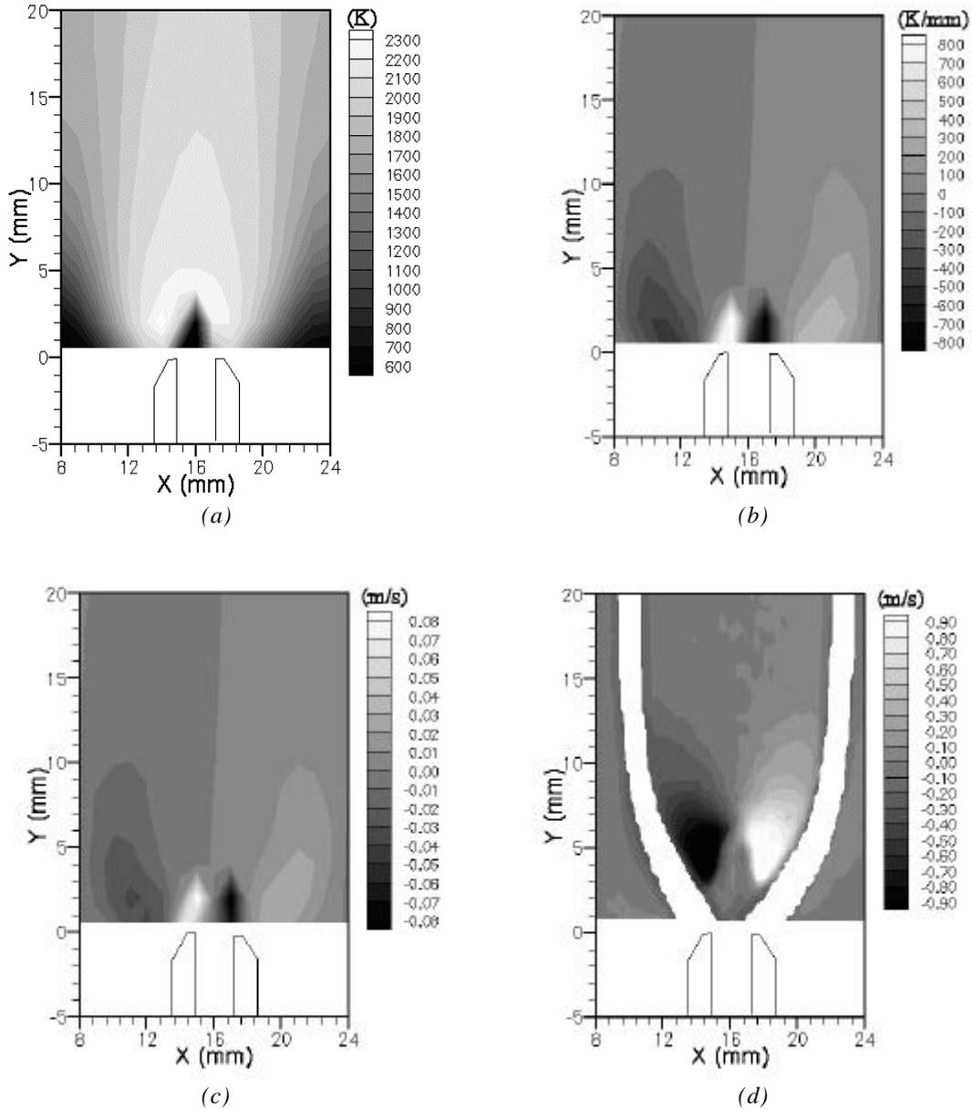
Figure 5: Gray-scale maps of temperature measured by fine wire thermocouples (a), of calculated horizontal temperature gradient (b), of calculated horizontal particle thermophoretic velocity, and of measured horizontal flow velocity  $V_x$  (d) for flame condition #2.
