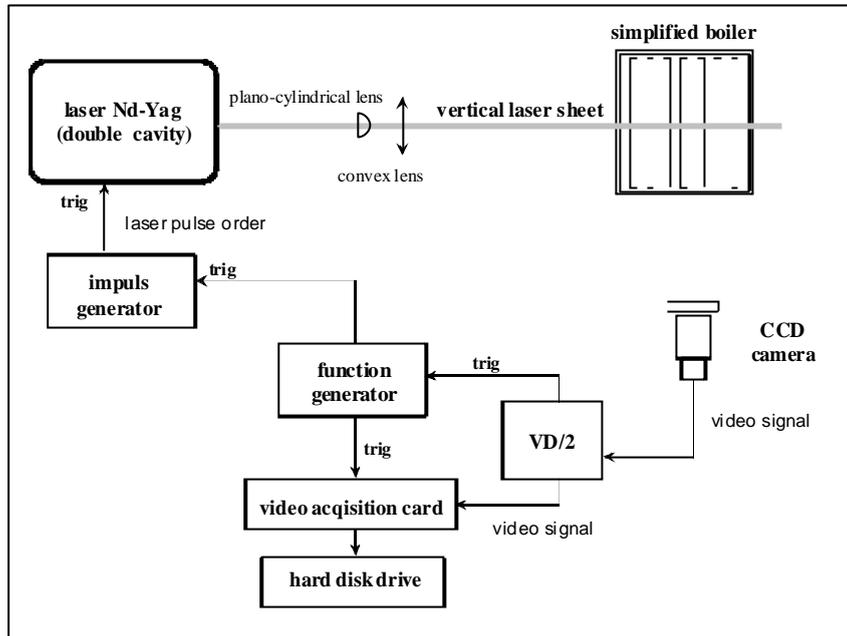
Figure 3: Schematic of the PIV system used in this study.
