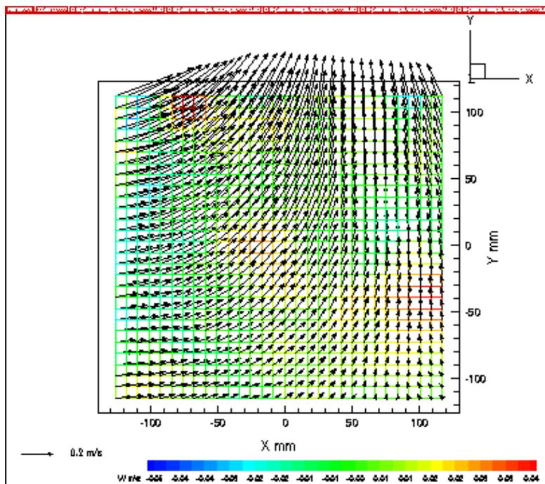
Fig. 9. Calculated 3-D velocity field as a three-dimensional vector plot underneath a broad-banded freak wave after two steps of pre-processing the images captured of both cameras
