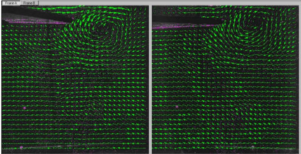
Fig. 7. Interaction of a regular intermediate water depth wave with a submerged horizontal plate.
