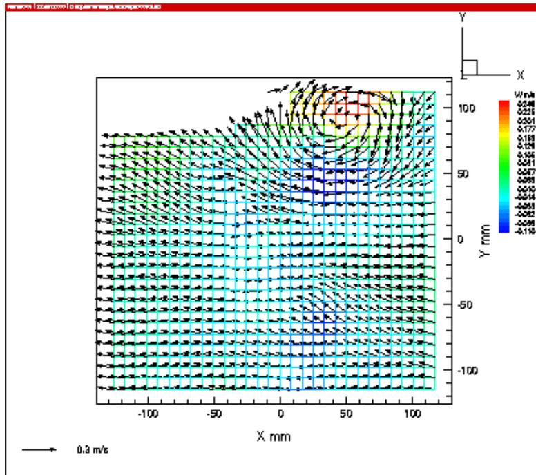
Fig. 8. 3-D Calculation of the velocity field: interaction of a regular intermediate water depth wave with a submerged horizontal plate as a primary breakwater
