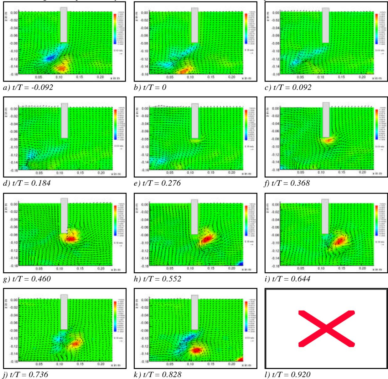
Fig. 6. Time history of the velocity field as vector plots and intensity of vorticity  $\omega$  in the disturbed wave field in constant time intervals  $\Delta t = 0.092$  s at discrete instants of time  $t/T$ , monochromatic intermediate water depth wave interacting with a semi-submerged vertical barrier
