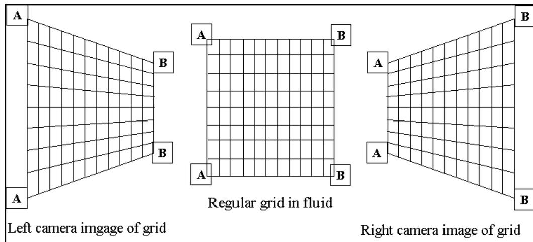
Fig. 4. Perspective effect due to camera tilt (see Bjorkquist, 1998)
