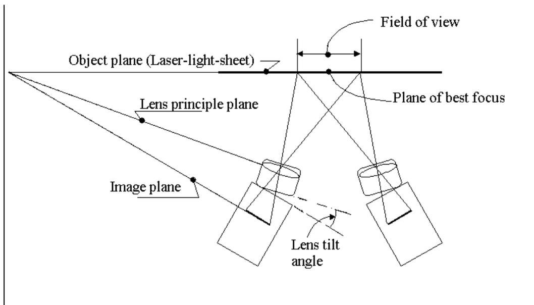
Fig. 3. Scheimpflug arrangement of the stereoscopic cameras (see Bjorkquist, 1998)
