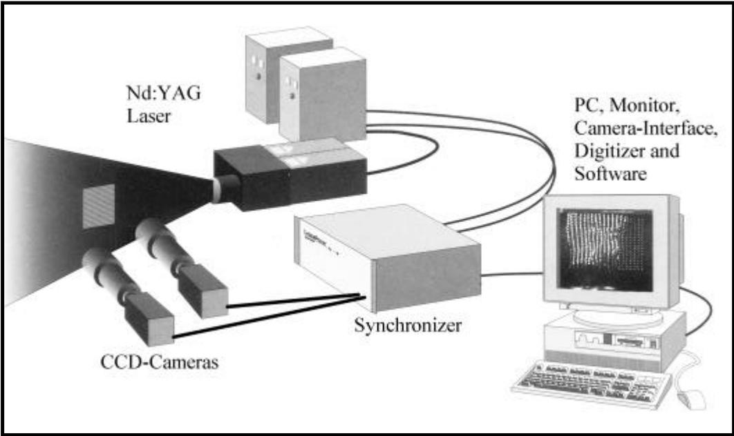
Fig. 1. Set-up of the stereoscopic PIV-system (schematically)
