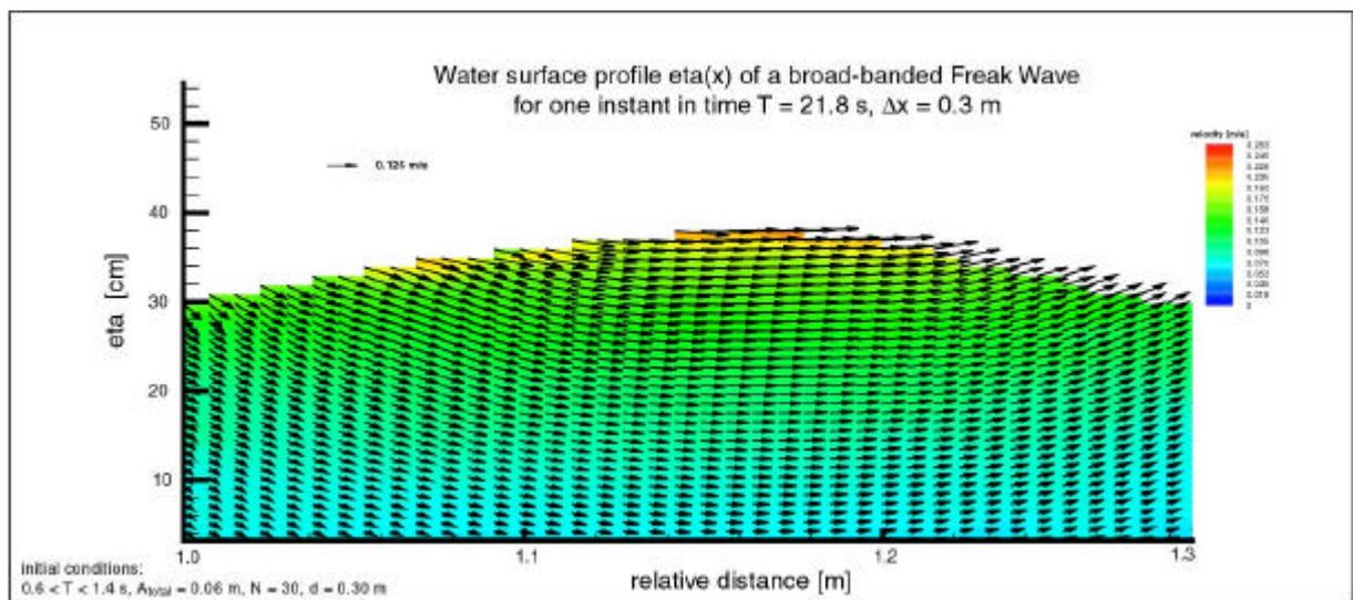
Fig. 10 Water surface elevation and velocity field as a three-dimensional vector plot underneath a broad-banded freak wave after post-processing
