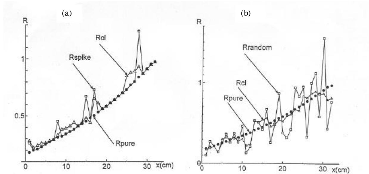
Fig. 5. Simulation results on the suppression/removal of noises for  $R$  signals by the wavelet transform method.
