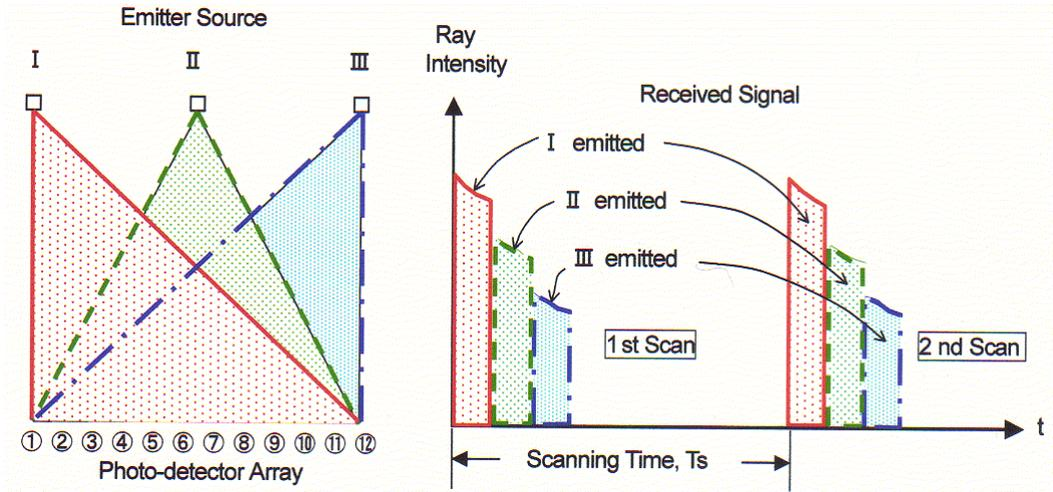
Fig. 2. Timing chart of emitters (laser diodes) and receivers (photo-detector array).
