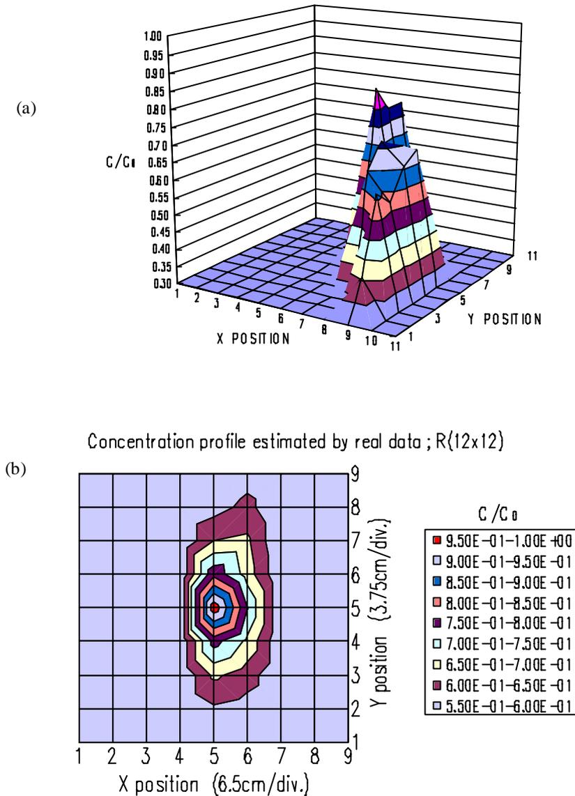
Fig. 4. Examples of 2-D concentration profile measured in a jet spray mist flow.
