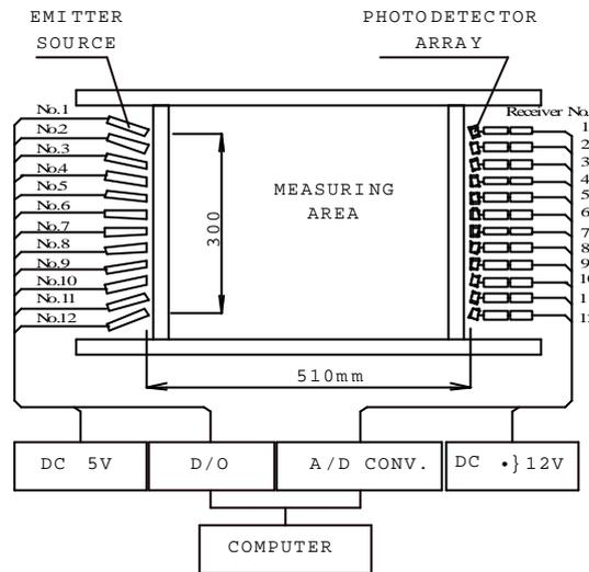
Fig. 1. Schematic diagram of the laser-sheet CT-scan type 2-D instantaneous concentration meter.
