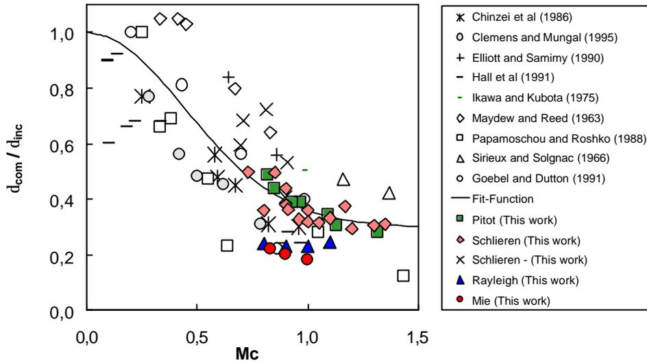
Fig 6: Normalized mixing layer growth rate in dependence of the convective Mach number  $M_c$ .
