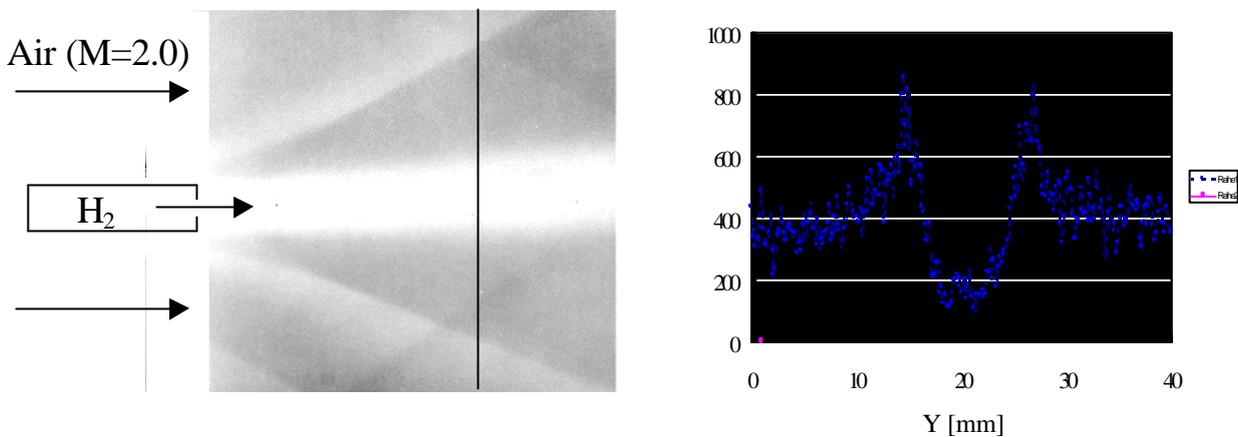
Figure 4: Averaged Rayleigh scattering image of the mixing layer zone in the vicinity of the plate injector and corresponding intensity profile
