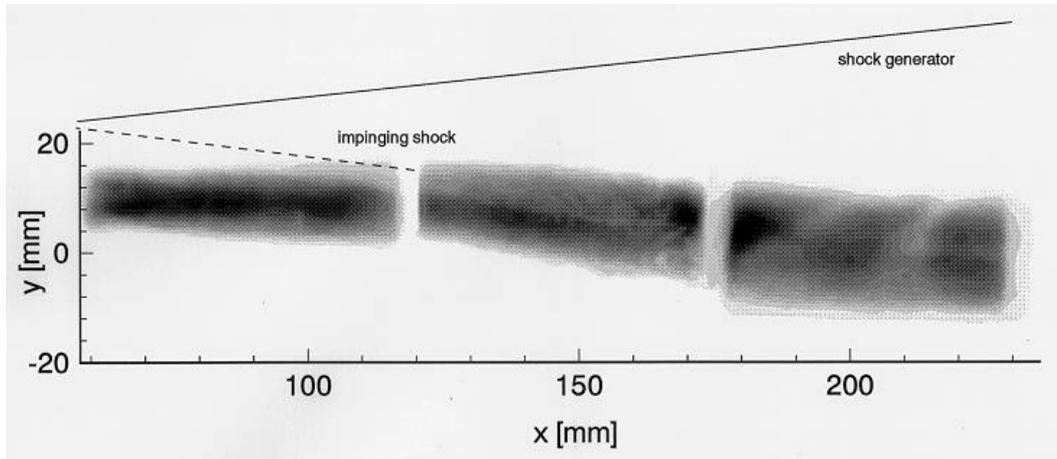
Fig 7: Mie scattering image of the mixing layer zone with shock impingement
