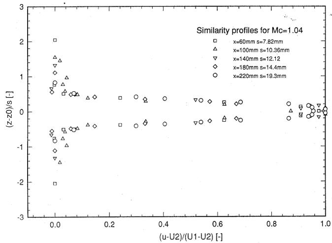
Fig. 3 Axial mean velocity profile and corresponding similarity profile for  $M_c=1.04$
