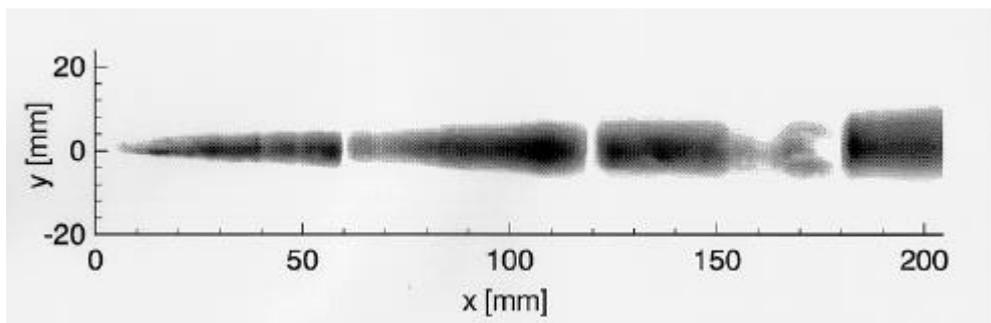
Fig 5: Averaged Mie scattering image of the mixing layer zone without shock impingement
