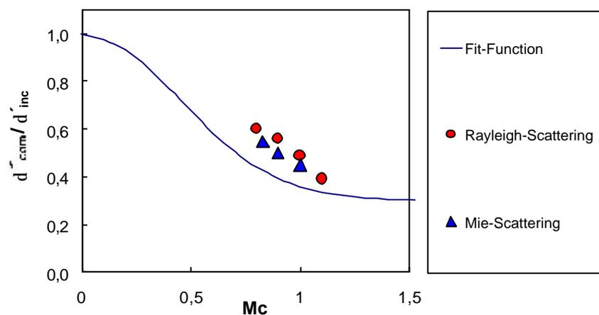
Fig. 8: Normalized mixing layer growth rate with shock impingement ( $\theta = 7^\circ$ )
