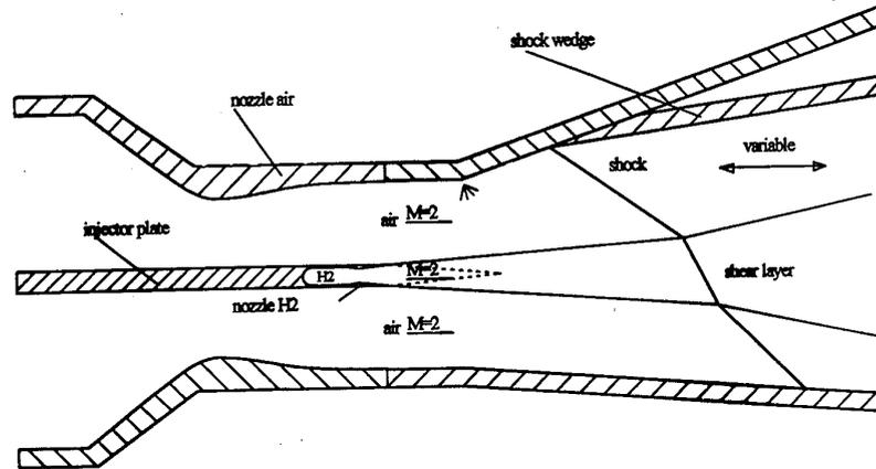
Fig. 1 Experimental supersonic model combustion chamber with plate injector
