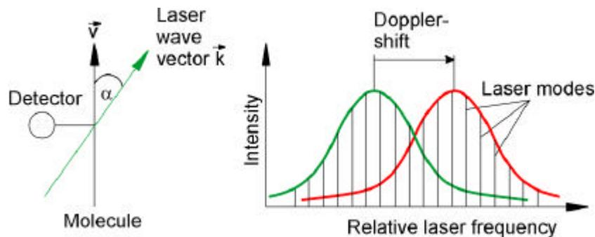
Figure 3. LIF velocity measurement using the Doppler-shifted absorption line.
