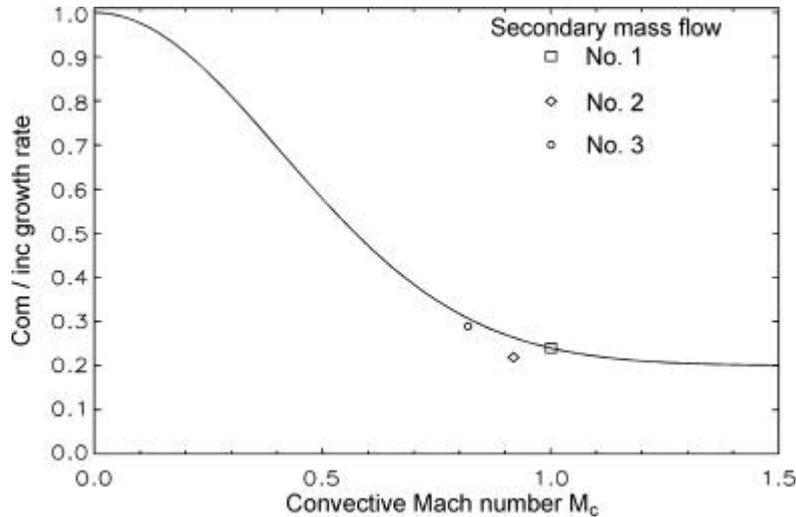
Figure 11. Comparison of the empirical curve for the plane free shear layer with the three measured growth rate ratios at convective Mach numbers of 0.82; 0.92 and 1.0.
