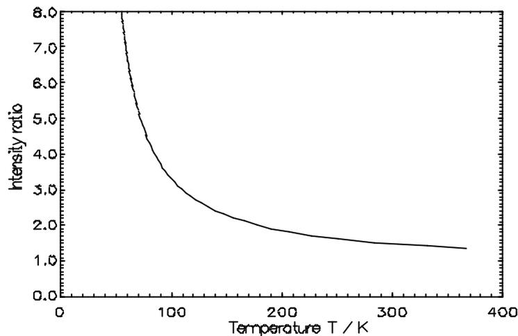
Figure 4. Calculated intensity ratio of the iodine absorption lines (P13/R15 to P103/P48) as a function of temperature.
