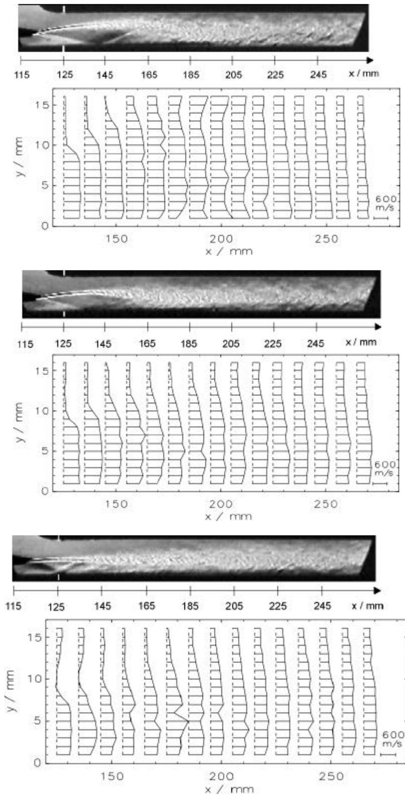
Figure 8. Schlieren pictures of the mixing chamber and corresponding one dimensional velocity distributions measured by the LIF system for secondary mass flows no. 1; 2 and 3 (from top to bottom).
