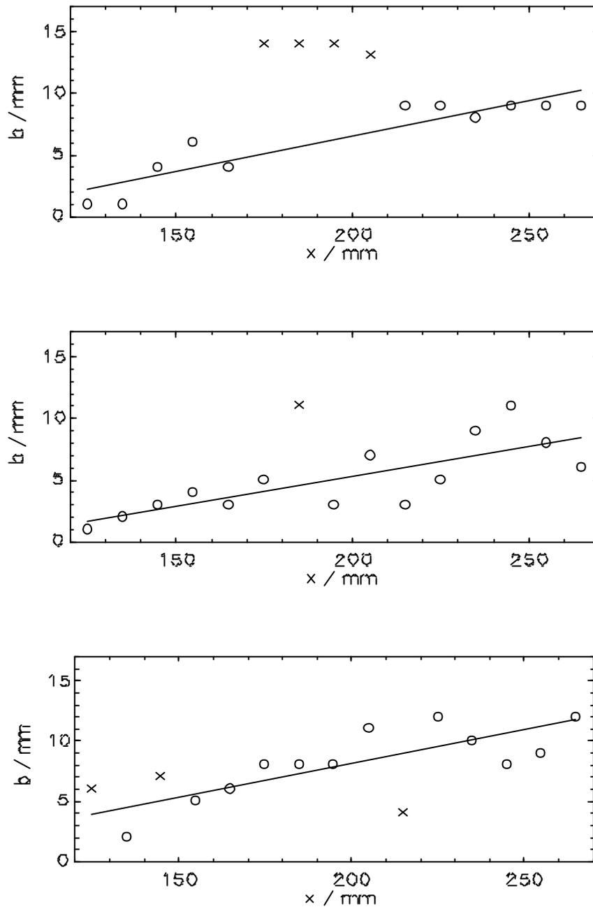
Figure 10. Streamwise evolution of the shear layer thickness in the mixing chamber. The datapoints were fitted by a straight line and the worst datapoints (crosses) were omitted for the fit. (Secondary mass flows no. 1; 2 and 3 from top to bottom).
