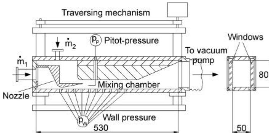
Figure 7. Supersonic ejector test section. All dimensions are expressed in mm.
