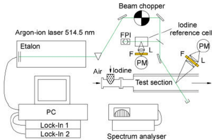
Figure 6. Set-up of the iodine LIF measurement system.
