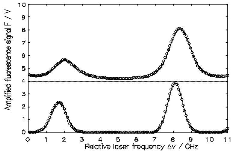
Figure 5. Iodine LIF spectrum measured at two different pressures: 7 kPa (upper) and 0.04 kPa (lower).
