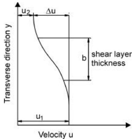
Figure 9. Definition of shear layer thickness.
