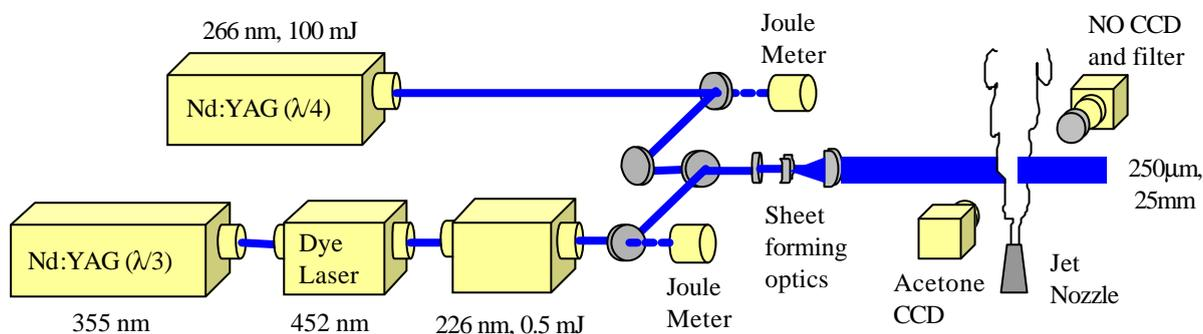
**Figure 1: Simultaneous NO and acetone PLIF lasers and optics.**
