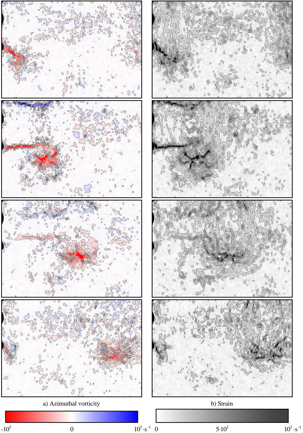
Figure 4. Vorticity and strain field calculated from four DPIV velocity maps. Phases equi-spaced along a forcing cycle. Flow comes from left to right. The nozzle exit lobes can be seen on the upper left side.
