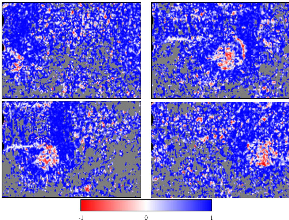
Figure 5. Local coefficient between azimuthal vorticity and strain calculated from four DPIV velocity maps. Phases equi-spaced along a forcing cycle. Flow comes from left to right. The nozzle exit lobes can be seen on the upper left side. The grey zones indicate zones where both the vorticity and the strain are negligible.
