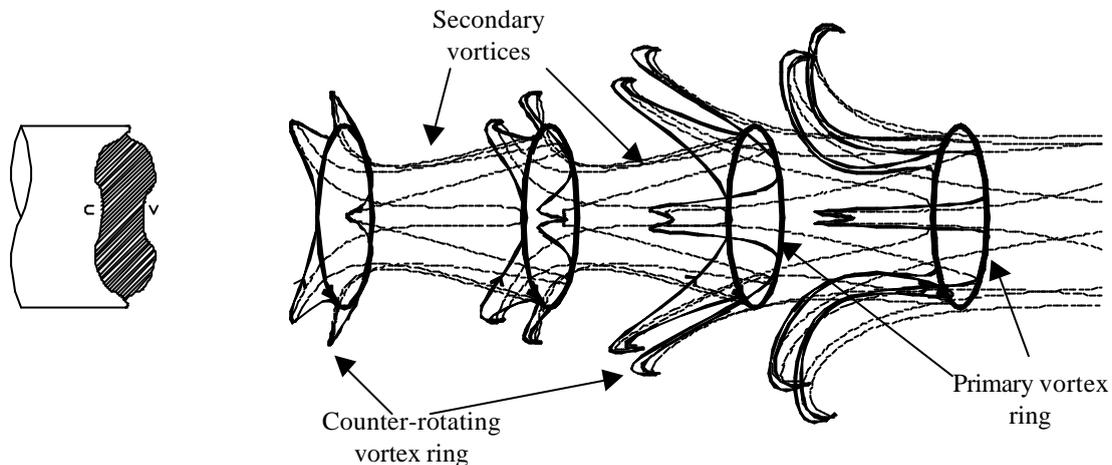
Figure 7. *Qualitative description of the near-field vortex dynamics for the high forcing amplitude case.*
