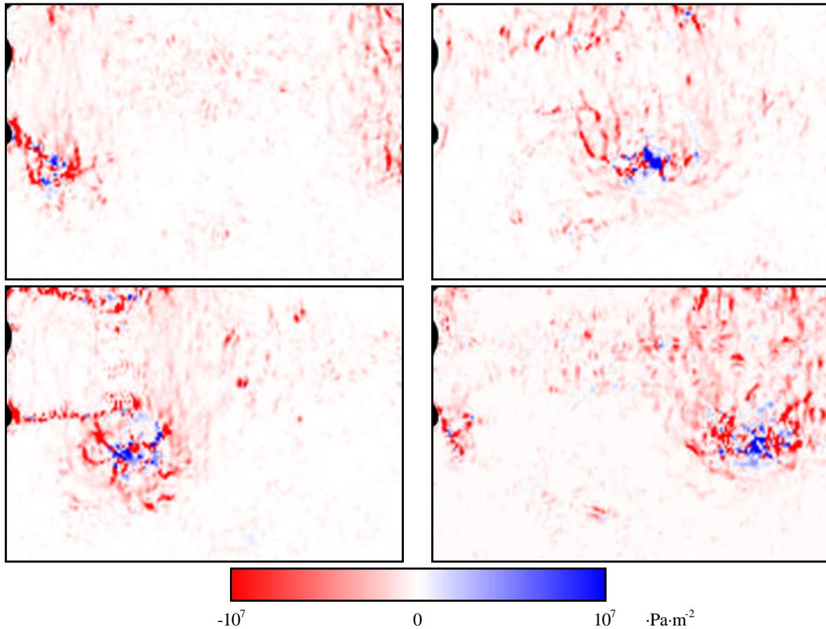
Figure 6. Laplacian of the pressure calculated from four DPIV velocity maps. Phases equi-spaced along a forcing cycle. Flow comes from left to right. The nozzle exit lobes can be seen on the upper left side.
