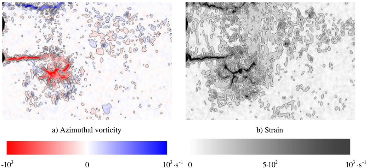
Figure 1. Vorticity field and strain field calculated from a DPIV velocity map. Flow comes from left to right. The nozzle exit lobes can be seen on the upper left side.
