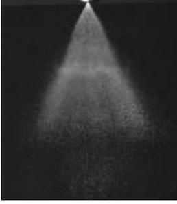
Fig. 7 Typical spray image at  $t=1.8\text{ms aSOI}$ ,  $P_{inj}=20\text{bar}$ .
