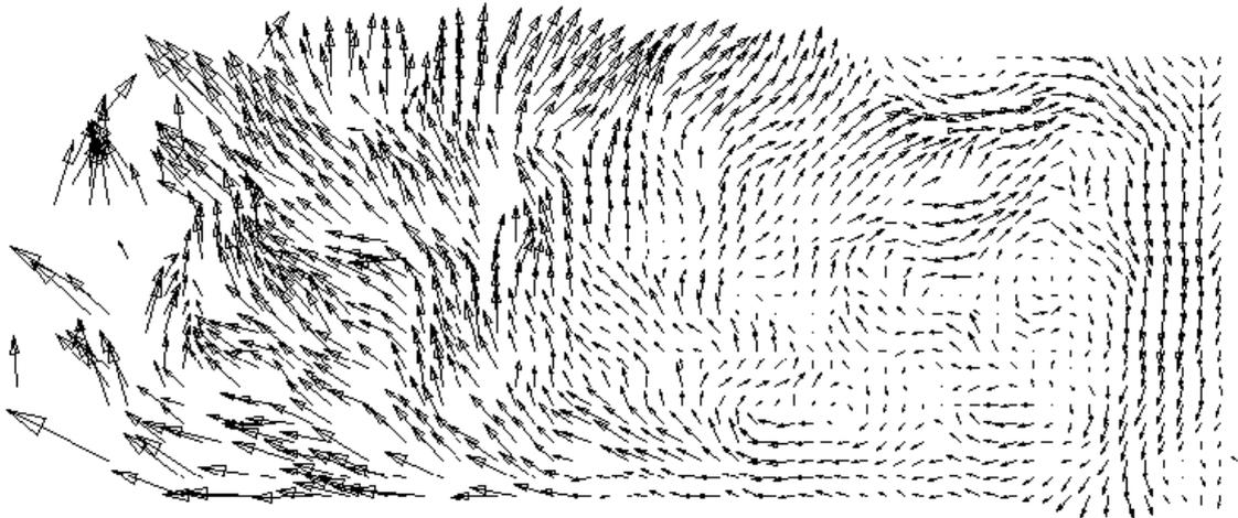
Figure 8. Instantaneous flow field of the continuous phase in the bubble column. Left side is close to the core, the right side is close to the wall. Missing vectors at the left side are caused by low scattering light intensity of the fluorescing tracer particles.
