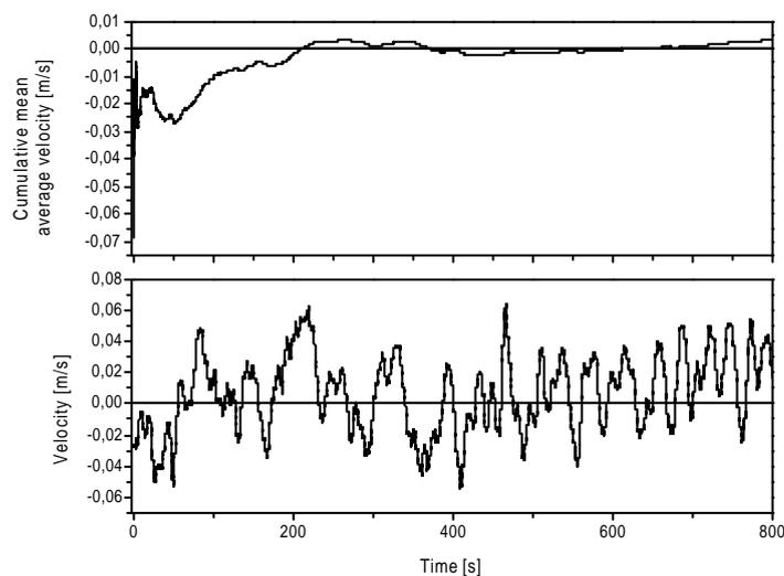
Figure 6. Time series of the axial liquid velocity measured with LDA and fluorescing tracer particles. The position of the measurement was 450 mm above the membrane aerator and the radial position was 50 mm. The mean flow velocity was 0.0035 m/s and the fluctuating velocity was 0.059 m/s. The upper graph shows the
