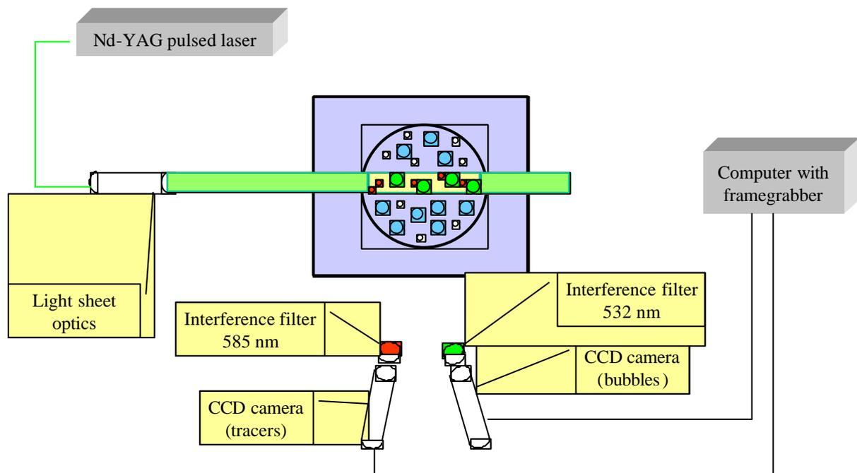
Figure 1: Two-phase PIV-system
