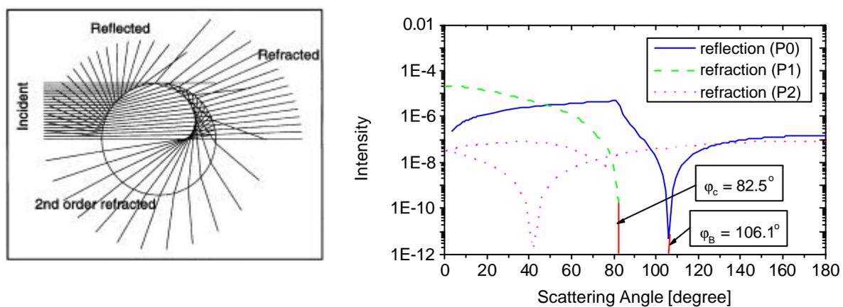
Figure 3: Air bubble in water. Left panel: ray tracings; Right panel: angular dependence of relative intensity for the different scattering components (logarithmic scale) for parallel polarisation.
