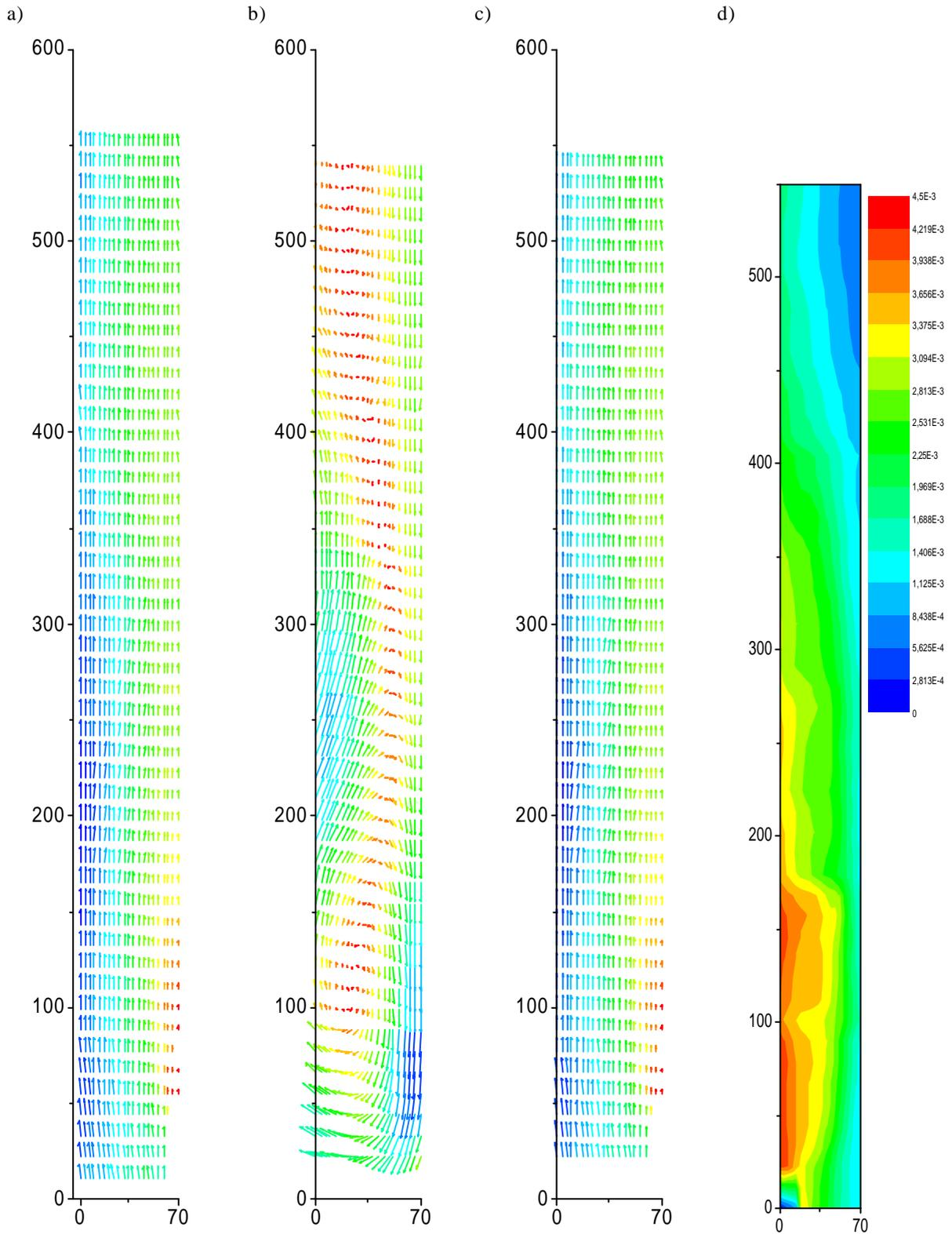
Figure 9. From left to right: vector plots of the averaged velocity fields of bubbles (a), liquid (b) and slip velocity (c); contour plot of the turbulent kinetic energy of the fluid (d). (The different vector plots do not have the same scaling.) The superficial gas velocity was 0.3 cm/s, the mean gas hold-up was 1,7 %, and the mean bubble diameter was 2 mm.
