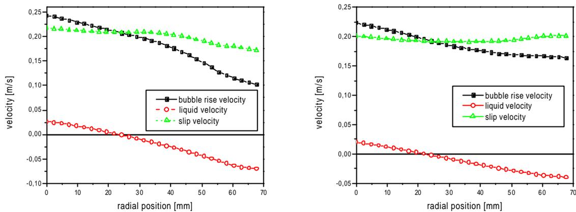
Figure 10. Profiles for the velocities of bubbles, liquid and slip velocity for different heights in the bubble column. Left: height=120 mm; Right: height=480 mm.
