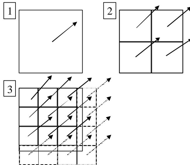
Figure 5. Scheme of the successive refinement of the interrogation area size. The size of the interrogation areas amount to 50\*50, 25\*25 and 15\*15 pixel, respectively (small structures of a flow like vortices were resolved only by small interrogation area sizes).
