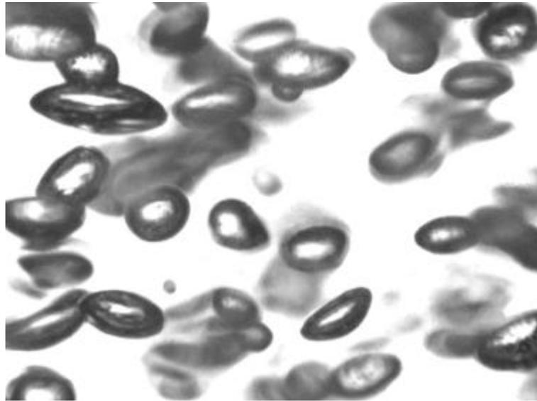
Figure 2. Typical image of bubbles in the core of the bubble column. The image was made by back lighting the scene with a pulsed LED-array. The focal length was 108 mm, and the aperture was completely open to provide a short depth of focus. The gas hold-up was 2,92%, and the mean bubble diameter was 3 mm.
