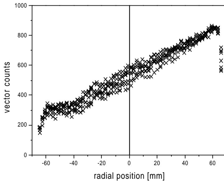
Figure 7. Influence of the optical path length of the laser light sheet on the number of validated vectors. (Cumulating of over 1000 vector-maps of bubble velocity in one section.)
