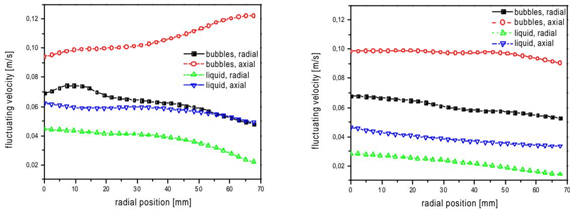
Figure 11. Profiles for the fluctuating velocities of bubbles and liquid for different heights in the bubble column. Left: height=120 mm; Right: height=480 mm.
