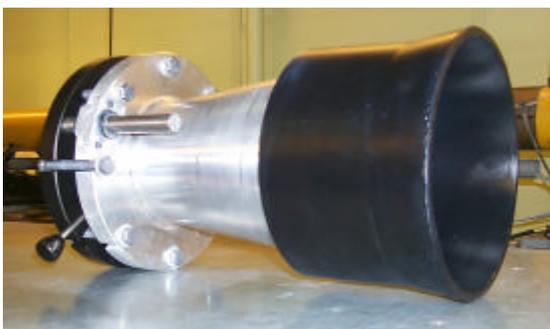
*Fig. 6. Conical non-reflected nozzle*
