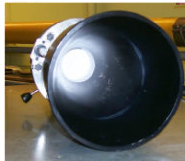
*Fig. 7. Inner non-reflected nozzle shape*
