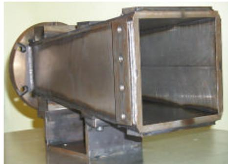
*Fig. 5. Square cross-section nozzle*
