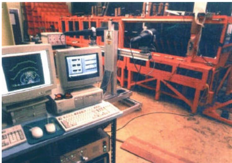
*Figure 1 Laser Doppler Anemometry measurement in the DERA Bedford Boundary Layer Tunnel.*
