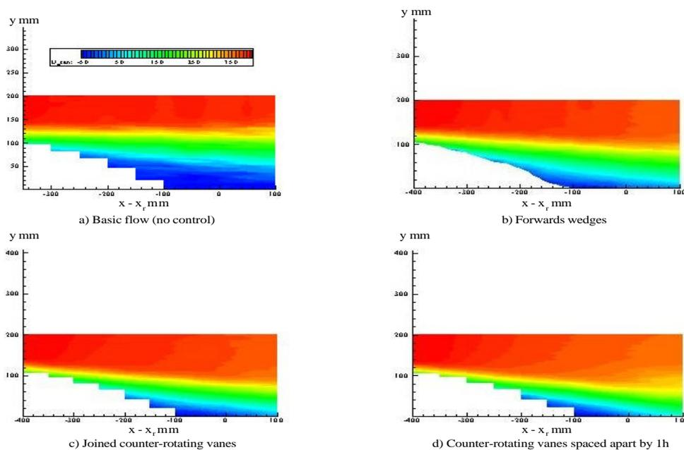
Figure 9 Contours of constant streamwise velocity in a vertical plane of symmetry over the separated flow.
