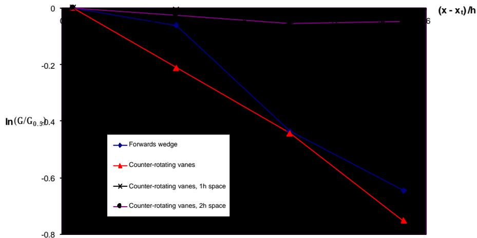
Figure 5 Decay of vortices downstream of various devices, zero pressure gradient,  $h = 30\text{mm}$ ,  $U_e \gg 30\text{m/s}$
