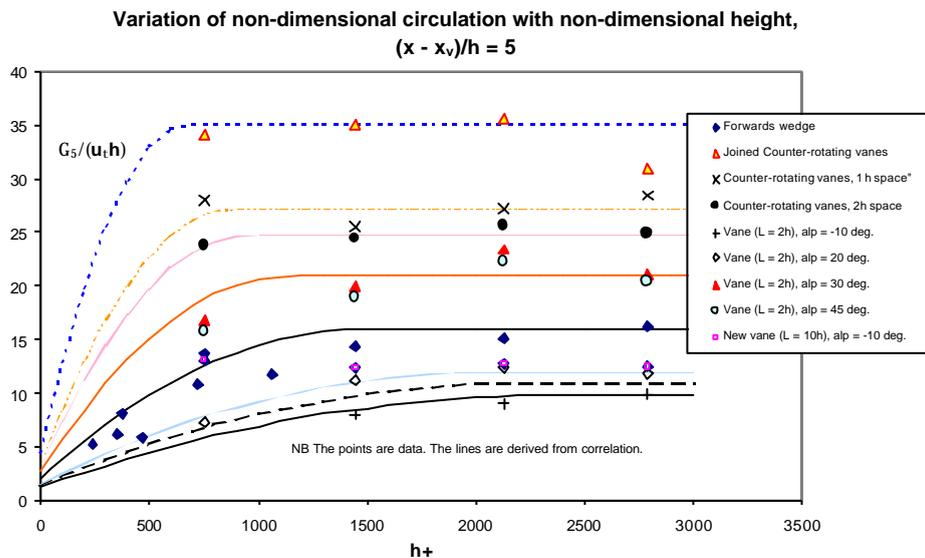
Figure 4 Non dimensional circulation versus non dimensional device height, zero pressure gradient
