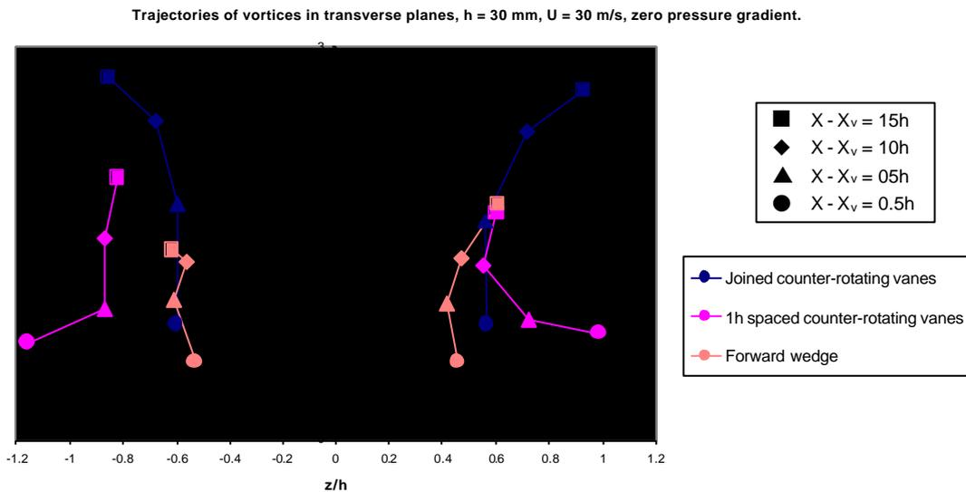
Figure 6 new vortex trajectory plot
