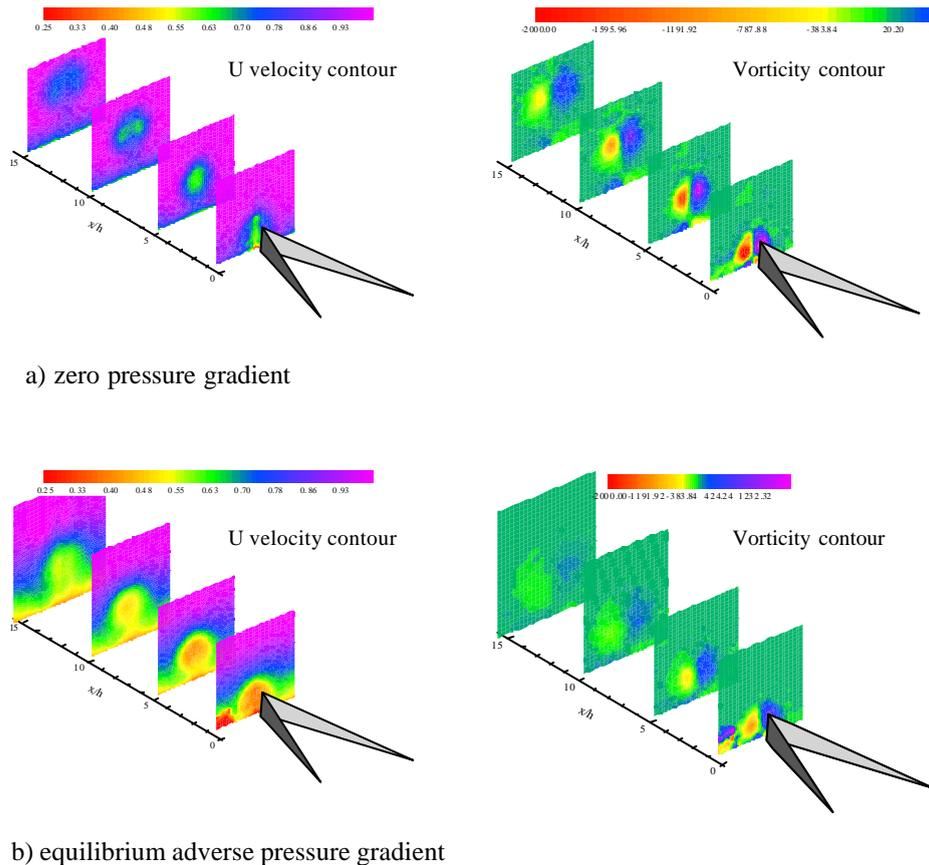
Figure 7 Downstream contours of  $U$  velocity and vorticity for the joined counter-rotating vanes in a) zero pressure gradient and b) equilibrium adverse pressure gradient.
