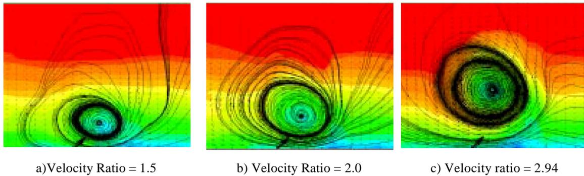
Figure 8 Typical effect on the position of the primary vortex with jet velocity ratio ( $U_{jet}/U_{\infty}$ ) at 20 jet diameters downstream. Contours of  $U$  velocity and secondary streamlines of  $v,w$ .
