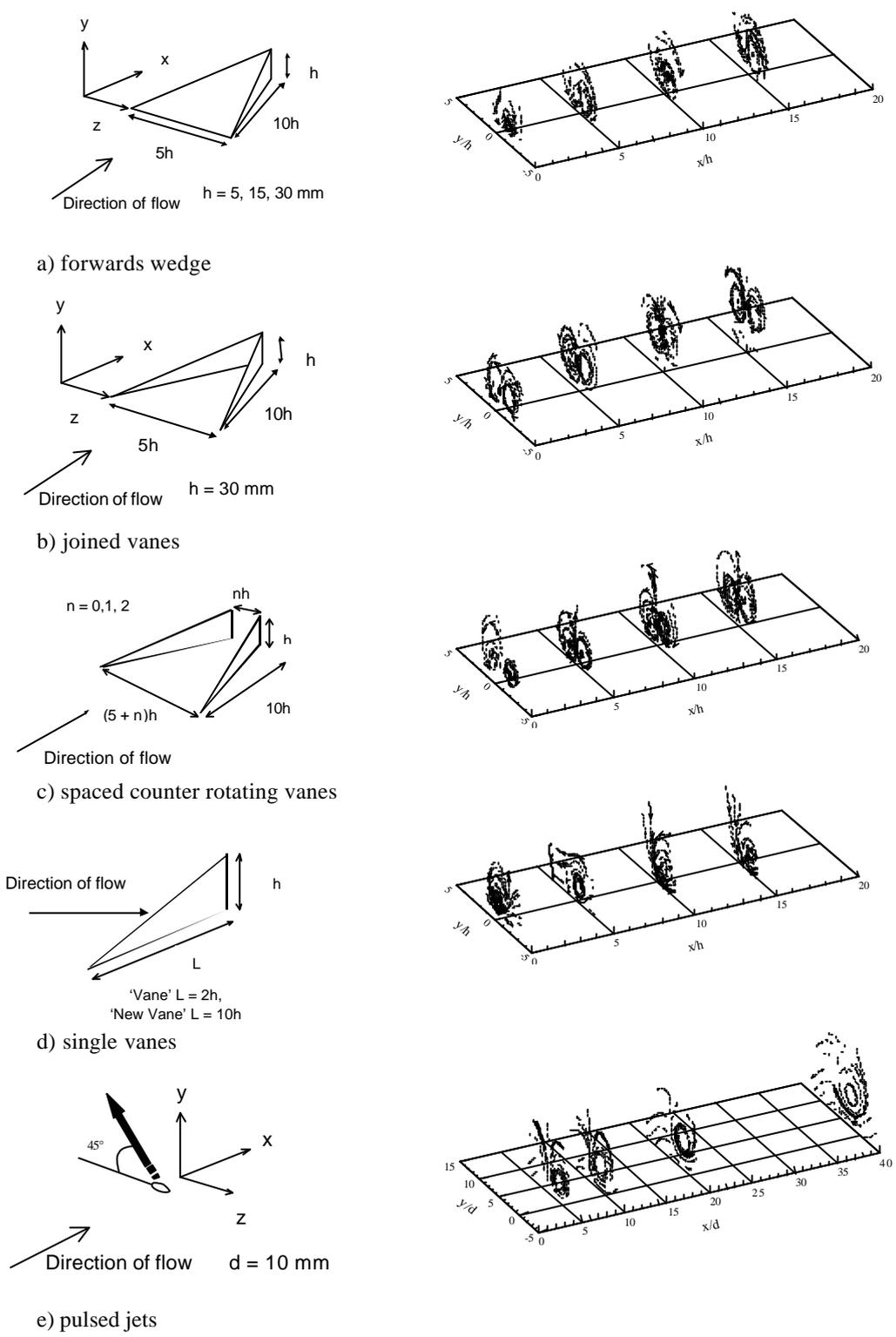
Figure 3 Devices tested accompanied by downstream progressions of cross-flow streamlines showing typical vortex structure.
