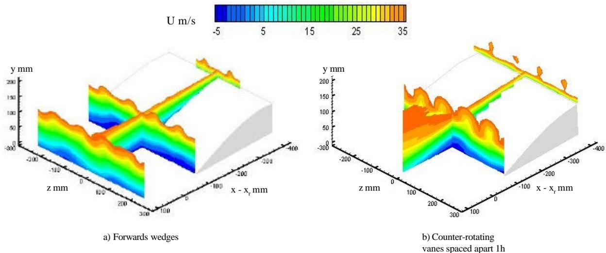
Figure 10 Isometric views showing contours of constant streamwise velocity in cross-flow planes.
