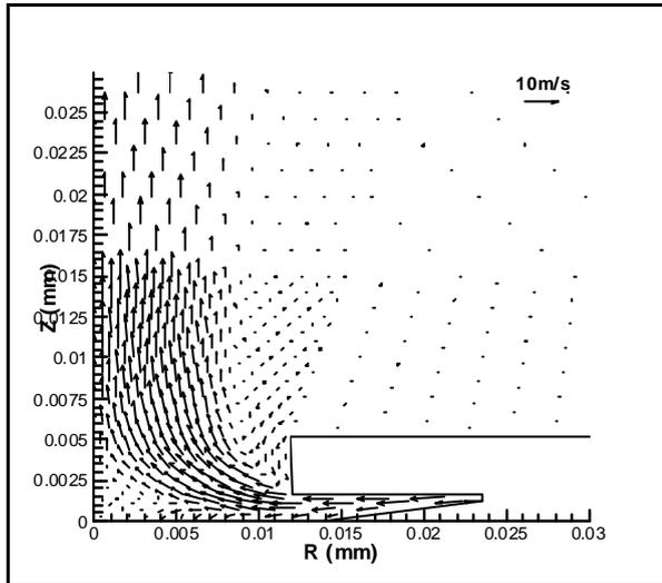
Figure 7. Velocity vectors for Axisymmetrical Argon injection at  $\theta=0^\circ$  - velocity: 11m/s
