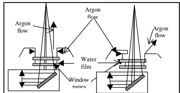
Figure 6. Left side: axi-symmetrical Argon injection
