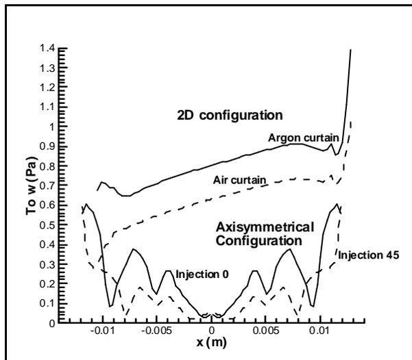
Figure 10. Wall shear stress along the window for same gas mass flow rates (Argon or air)
