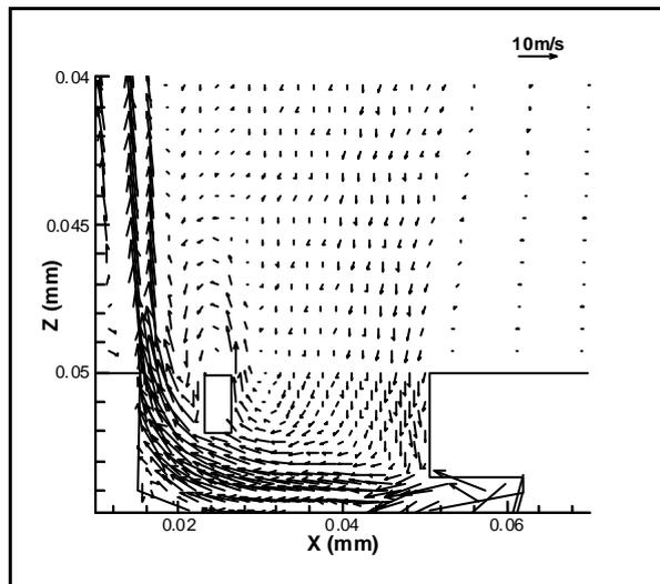
Figure 9. Velocity vectors for on-side Argon injection at  $\theta=45^\circ$  velocity: 30m/s
