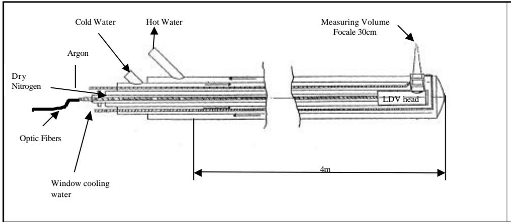
Figure 5. Scheme of the water cooled LDV probe
