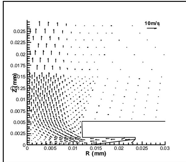
Figure 8. Velocity vectors for Axisymmetrical Argon injection at  $\theta=45^\circ$  - velocity: 11m/s
