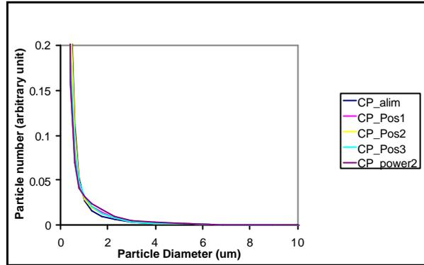
Figure 12. Particle distribution in number for different PC jet locations.
