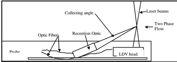
Figure 2: Scheme of the Intrusive Phase Doppler Granulometer
