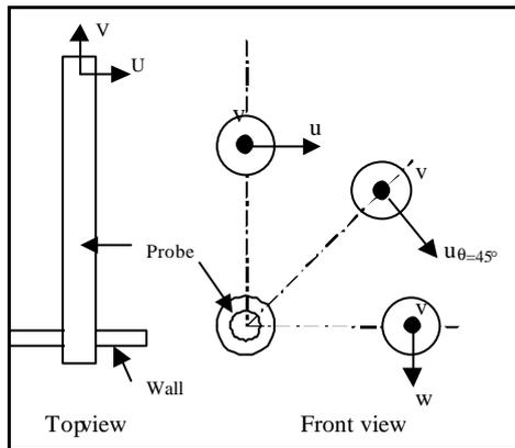
Figure 4: Measured velocity components as probe angle.  $v$  is the velocity component parallel to the probe axis
