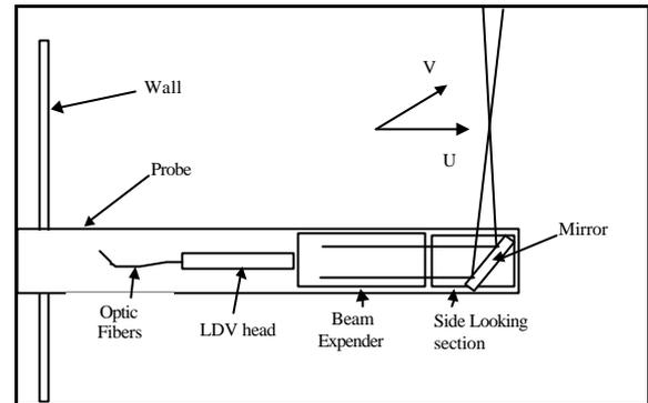
Figure 3. LDV System with Beam Expander and Side Looking Section
