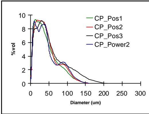
Figure 11. Particle distribution in volume for different PC jet locations.
