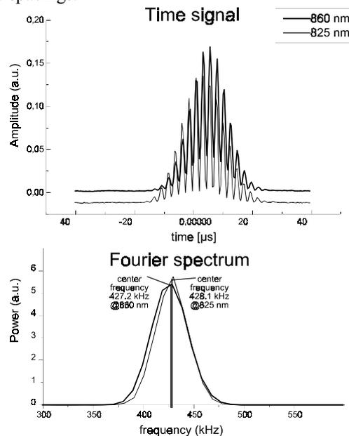
FIG. 11. Measuring results from the two channels for a single longitudinal position ( $z=z_c-0.05\text{mm}$ ) Top: Burst time signal; bottom: FFT spectra of the Doppler frequencies.
