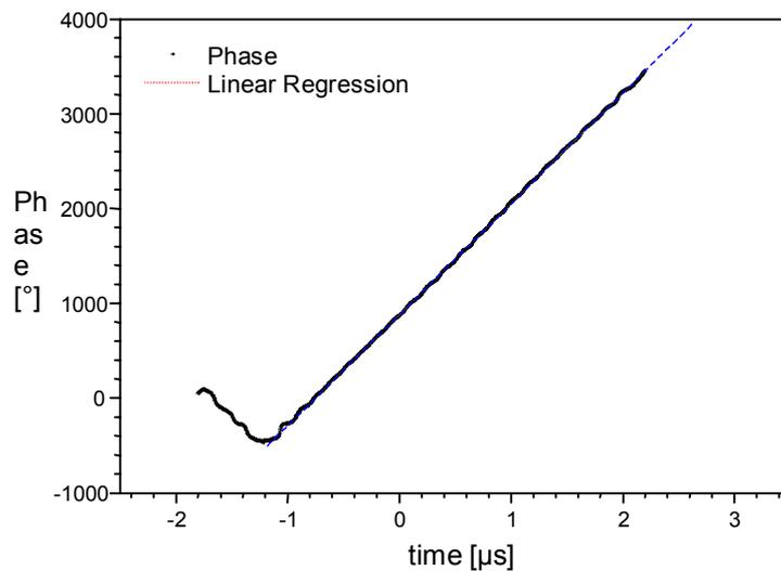
Fig. 8: Demodulated phase of the quadrature signal pair from Fig. 7. Using a straight regression curve, their slopes give the amount of the averaged Doppler frequency and the direction of motion.
