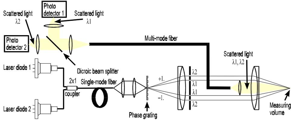
FIG. 10. Arrangement of the proposed LDV system, yielding a spatial resolution. Two laser diodes of different emission wavelengths are employed to generate the different fringe systems. The back-scattered light is chromatically separated into two detection channels. The evaluation of the two Doppler burst signals by FFT technique allows a determination of the  $x$ -velocity component  $v_x(z)$  as a function of the  $z$ -position of the tracer particle trajectory.
