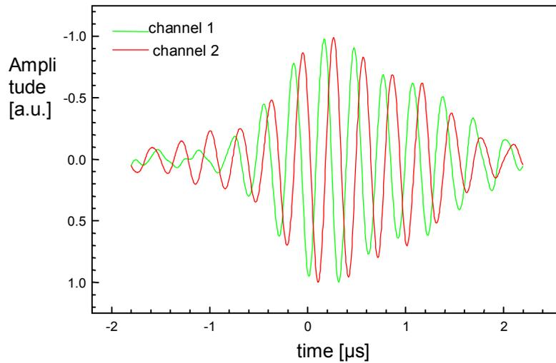
Fig. 7: Band pass filtered quadrature signal pair, compare Fig. 5.
