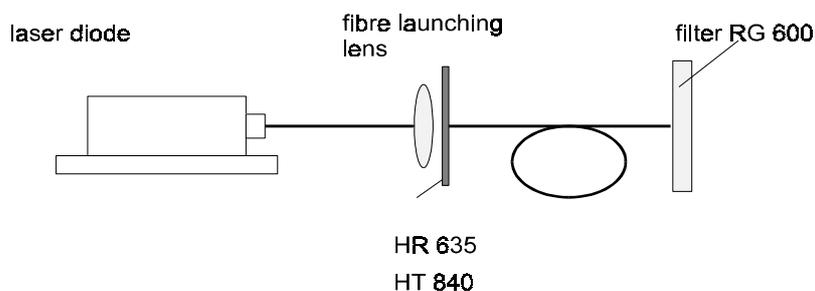
Fig. 3. Principle of a diode-pumped fibre laser, emitting at two wavelengths. A Pr/Yt doped glass fibre is pumped by a mopa diode laser of 840nm wavelength. Due to up-conversion processes, an emission wavelength of 635nm is achieved, see Zellmer et al. 1999.
