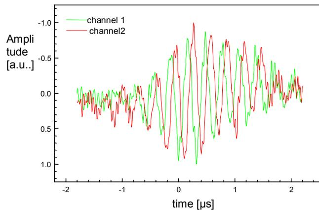
Fig. 5: High-pass filtered quadrature signal pair for one moving direction
