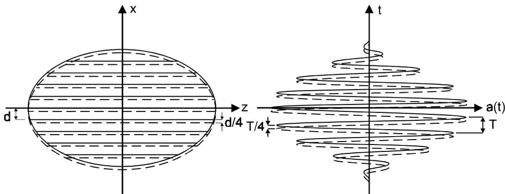
Figure 2: Principle of the two-colour directional discrimination technique. A pair of fringe systems with equal fringe spacing but a quadrature phase shift of  $90^\circ$  is generated in the measuring volume. The generated signal pair in the base band has a phase shift of  $\pm 90^\circ$ , where its sign is dependent on the direction of the particle movement.
