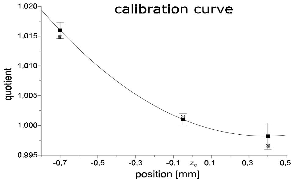
FIG. 13. Experimental calibration curve. The quotient of the fringe spacings  $q=d_2/d_1$  as a function of the z-position is shown. The validation range of the spatial resolved velocity measurement results to  $z_c-0.8\text{mm}$  to  $z_c+0.4\text{mm}$ . The error bars depict the accuracy of the measured quotient  $q$  at three arbitrary z-positions (5 repeated measurements).
