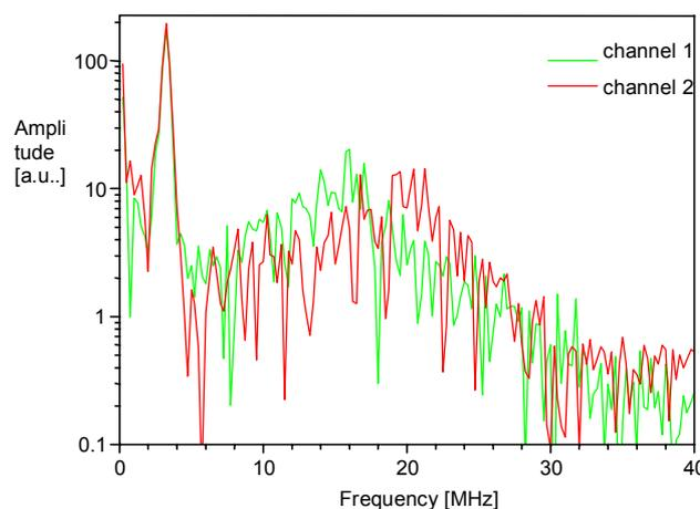
Fig. 6: FFT spectrum of the measuring signal from Fig. 5.
