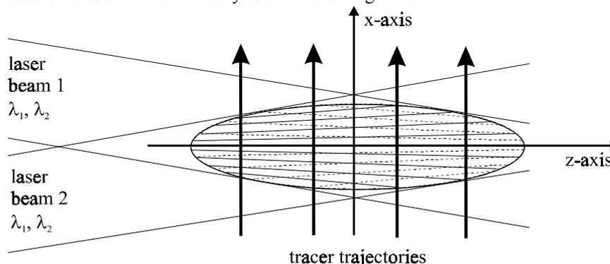
Fig. 9. Concept of the spatial resolution principle. Two fringe systems are generated with different spatial dependence of their fringe spacings along the  $z$ -axis. Their separate evaluation allows a spatial-resolved velocity measurement  $v_x(z)$ .
