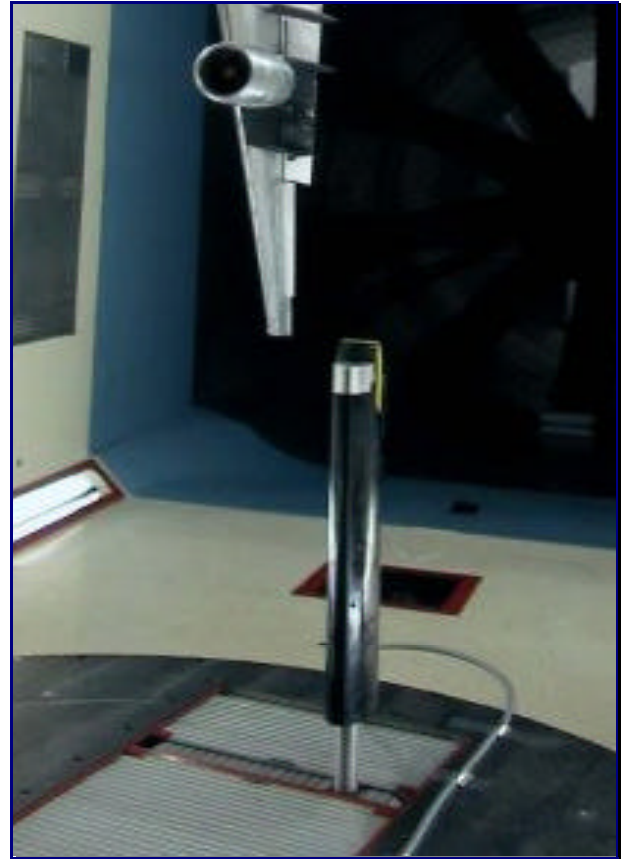
Fig. 3: 2D laser Doppler velocimeter mounted on a 3D traversing unit
