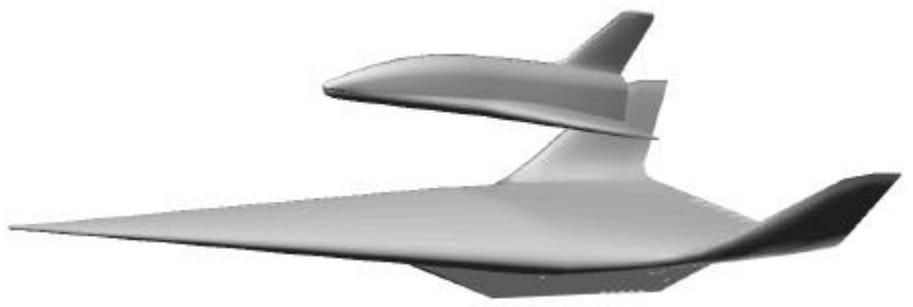
*Figure 2: Two-stage-to-orbit vehicle with the first stage ELAC and the second orbital stage EOS. ELAC is designed as a hypersonic flight vehicle, which takes off horizontally and flies up to an altitude of  $\sim 30$  km, where it comes up to  $Ma = 7$ .*
