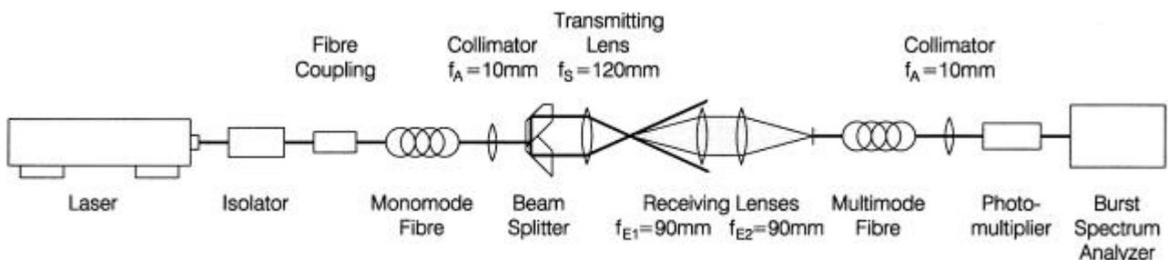
Fig. 5 Schematic view of the optical arrangement
