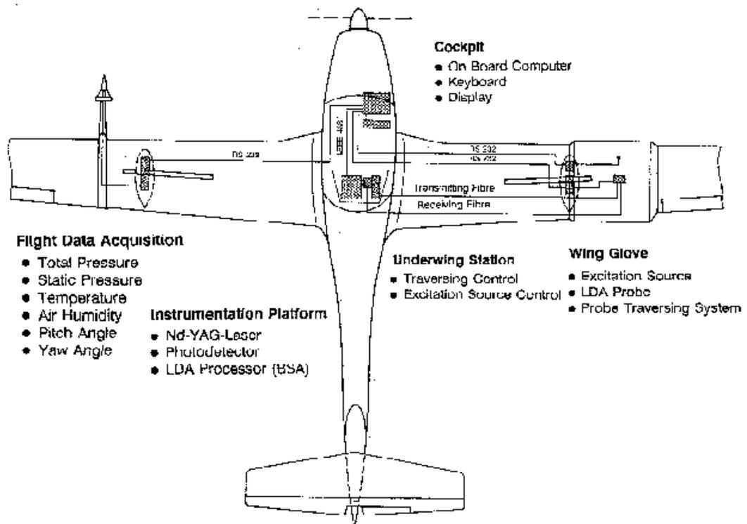
Fig. 8 Arrangement of instrumentation on the test aircraft
