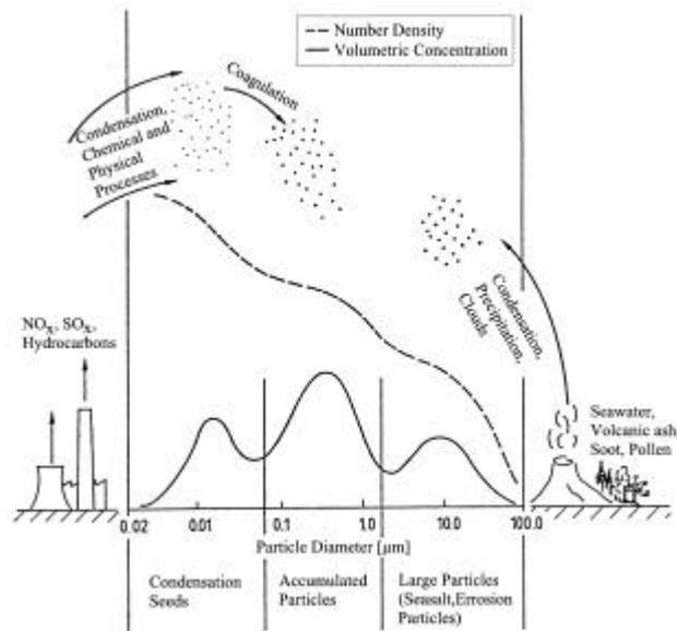
Fig. 3 Origin and size distribution of atmospheric particles
