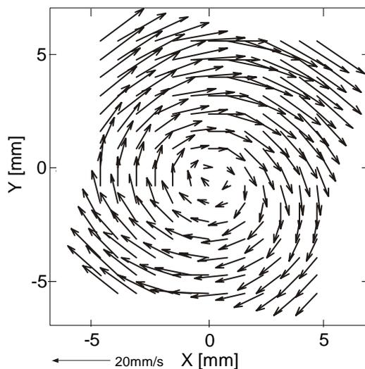
Figure 11 Mean Velocity Map of Moving Particles on a Turn Table(33rpm)
