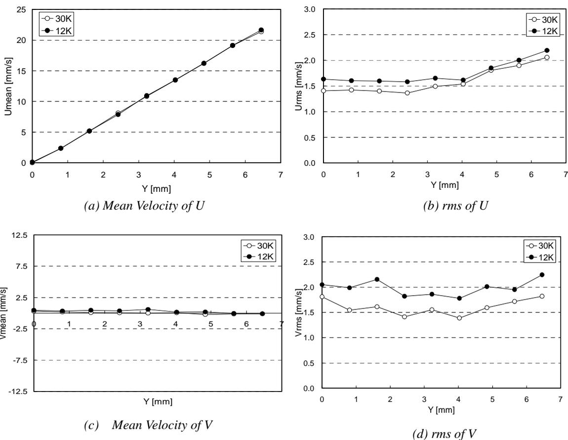
Figure 12 Mean Velocity and RMS of Cross-Correlation PIV at  $X=0\text{mm}$
