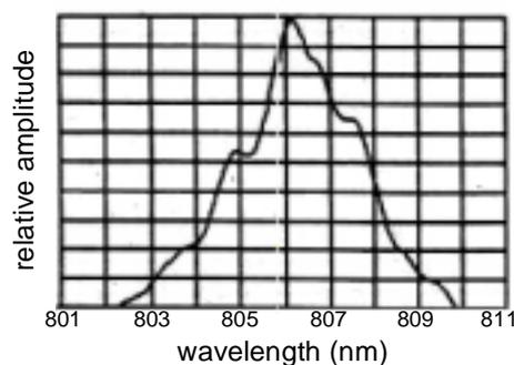
Figure 4 Wavelength Distribution of Laser Diode
