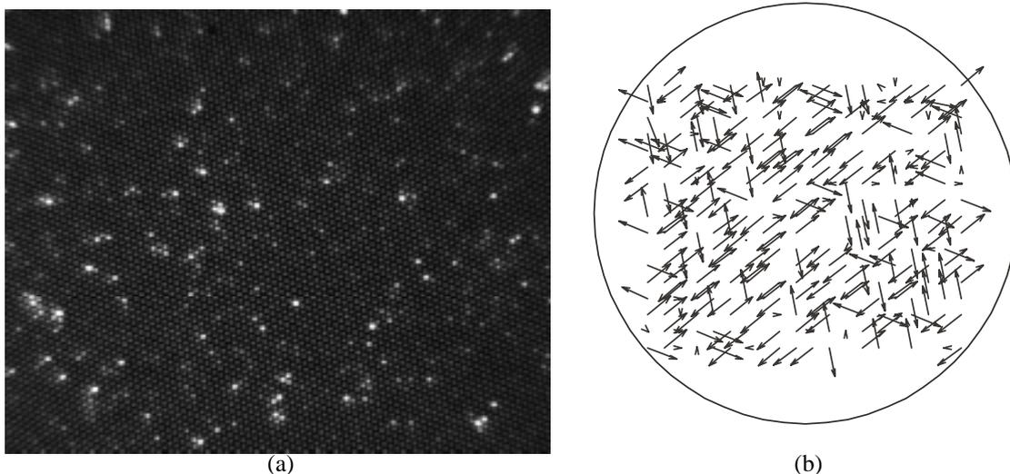
Figure 9 Partial Particle Image through a Fiber Bundle and Result of Conventional Cross-Correlation
