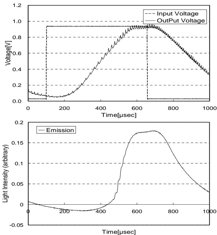
Figure 5 Pulse Delay Characteristics of Laser Diode
