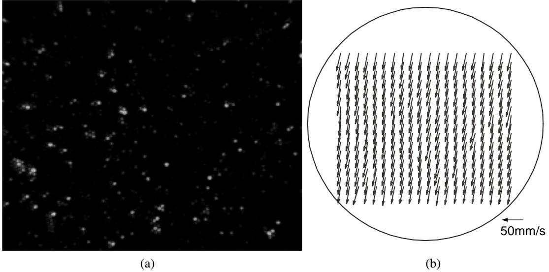
Figure 10 (a) Particle Image Eliminated a Pattern of Fibers and (b)Vector Map
