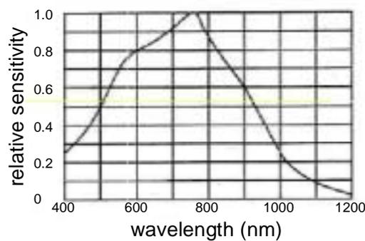
Figure 6 Spectral Sensitivity Characteristic of Near Infrared CCD Camera
