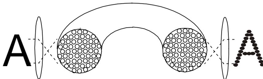
Figure 7 Directly Transformation of an Image Optical Fiber Bundle and Transferred Image of Lower Resolution
