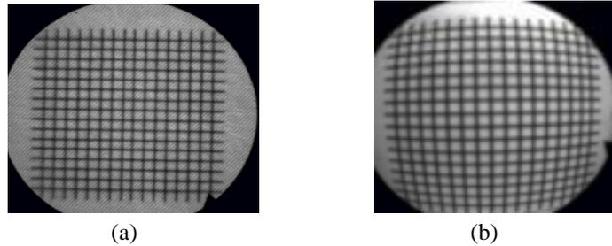
Figure 8 Distortion of Image (a) 10 degrees of view (b) 40 degrees of view
