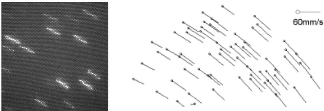
Figure 2 Particle Streak Image and Velocity Vectors
