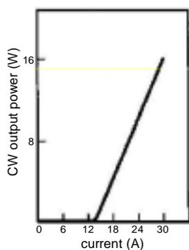
Figure 3 Light vs. Current Characteristics
