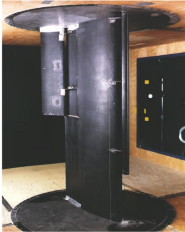
Figure 10. Three-element wing with part-span high-lift system in 7- by 10-Foot Wind Tunnel.
