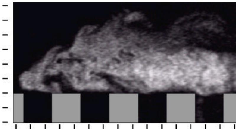
19 mm roughness element array. Scales shown are in 1 cm increments.
