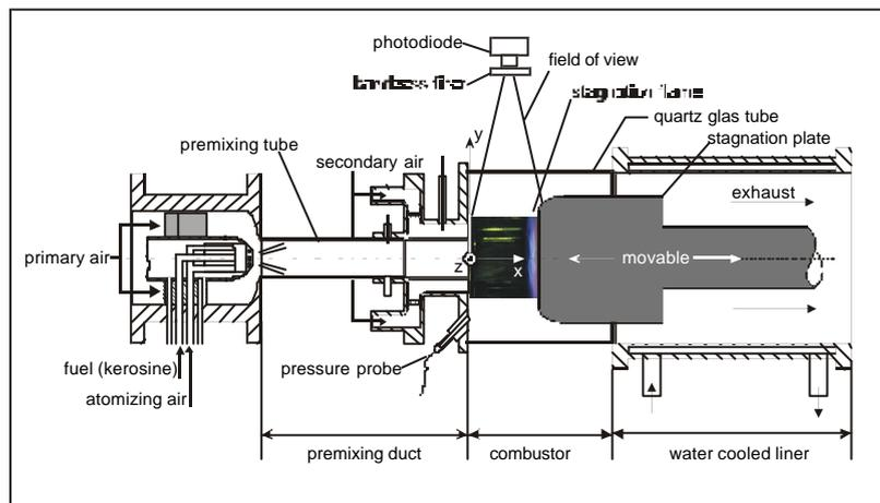
Fig. 1: Sketch of the experimental setup
