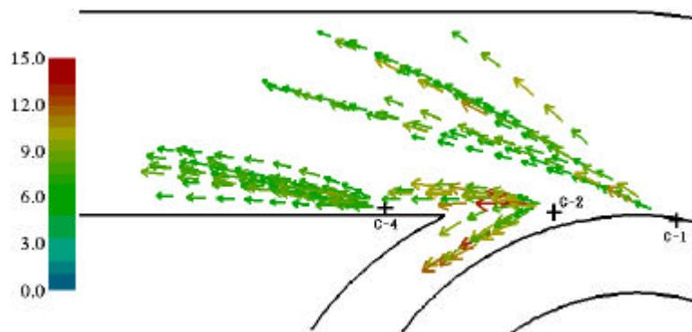
Fig.1 Velocity vectors illustrating unstable flow, Volute C,  $f=0.27$
