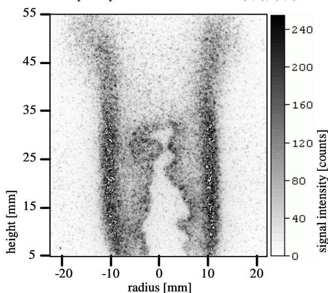
**Fig. 1: OH LIF single shot measurement in a methane/air Bunsen burner flame. Excitation frequency at  $38322 \text{ cm}^{-1}$ .**
