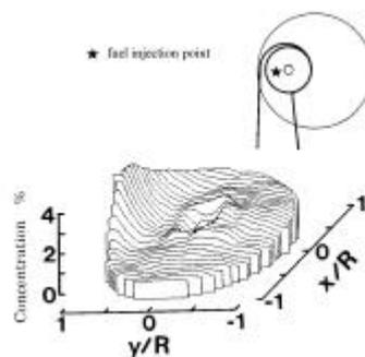
Fig.1 Fuel concentration of the swirl port with fuel injected at the intake valve ( $z=70\text{mm}$ ).
