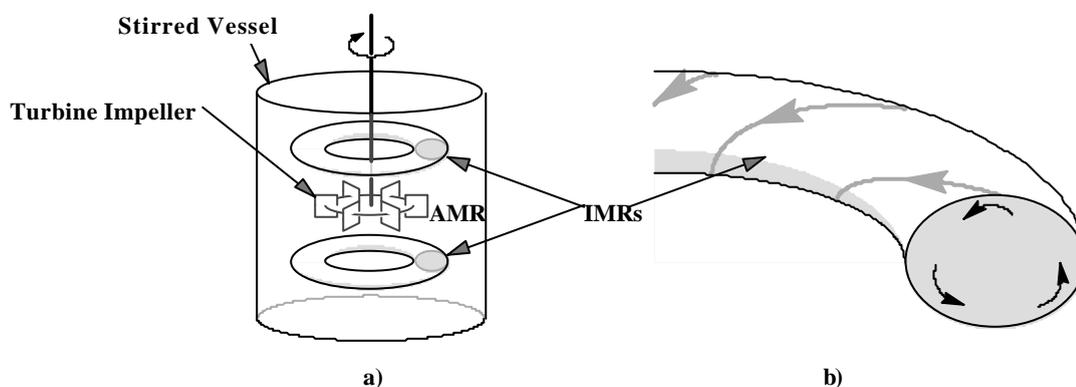
Fig. 1. Schematic picture of IMR in the stirred vessel
