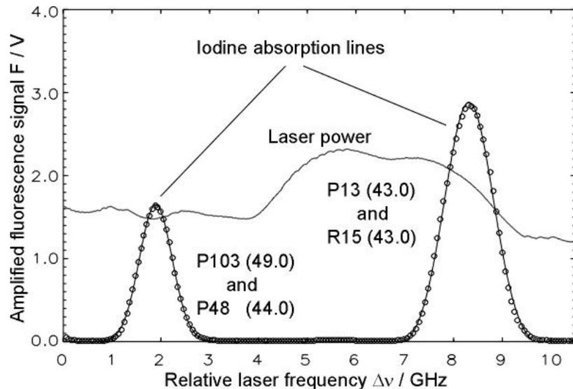
Figure 1. Measured iodine absorption spectrum by tuning a 514.5 nm single mode argon-ion laser. The absorption lines are assigned by their rotational and vibrational quantum numbers. The measured data points are fitted by a Gaussian function. The laser power used for normalisation is also recorded.
