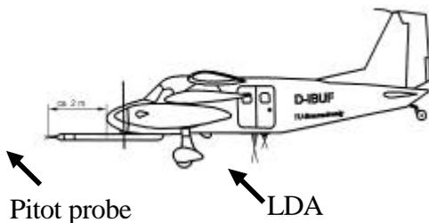
Fig. A: Side view of DO-128 research aircraft, indicating measuring locations.
