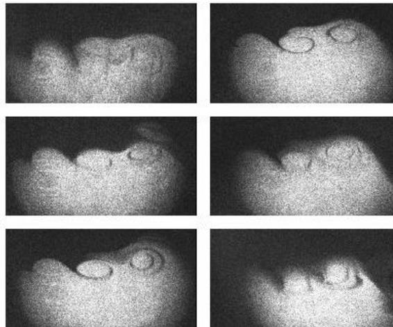
**Fig. 1** Plane-wise sampling of a three-dimensional vortex structure in the boundary layer between an axisymmetric jet and surrounding air. Field of view  $44 \times 70 \text{ mm}^2$ , at a distance 30 mm downstream of the nozzle, image planes equally separated over 35 mm depth. The lower field boundary coincides with the nozzle axis.
