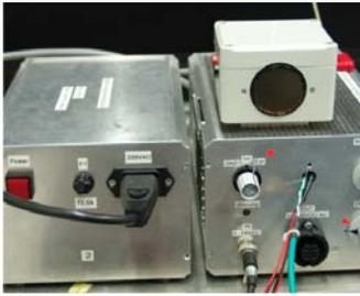
**Fig. 2.3** CUT (SensComp, Inc.) used in the present setup and its power supply (self-made). Transducer diameter  $\approx 40$ mm
