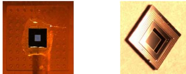
**Fig. 4.2** Sensor with roughened top diaphragm surface and inserted in a 0.25 mm thick, laser structured Kapton foil (left), Exposed rear side of the sensor with cavity and rear side of the diaphragm (right)
